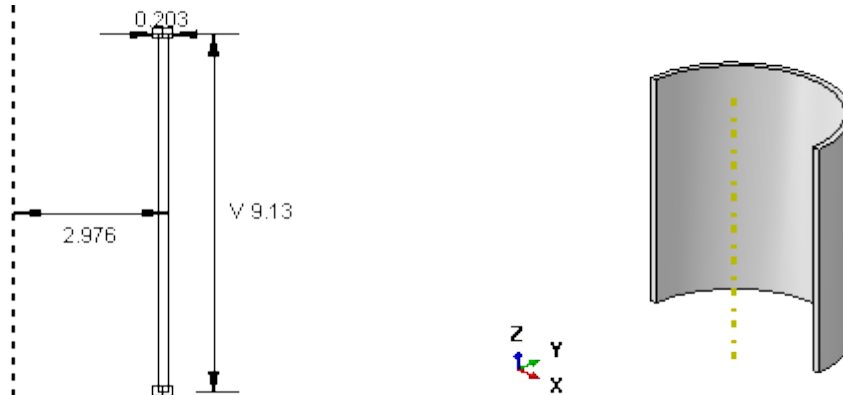
Figure 5.2: Cross-section dimensions for sleeve, given in mm (left) and modeled component produced by revolution (right).
