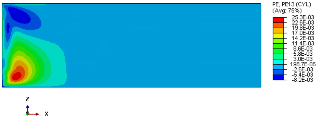
Figure 6.8: The r - z plastic shear strain fields for the “baseline” case.
