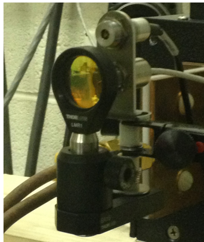
Figure 2-13: Infrared thermometer with laser-sighting tool and focusing lens
