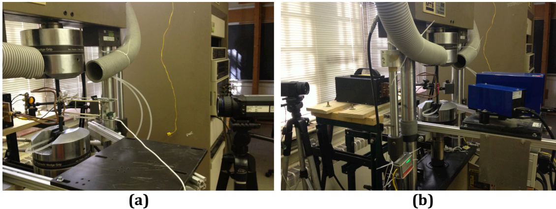
Figure 3-1: Test setup with mechanical and laser extensometer
