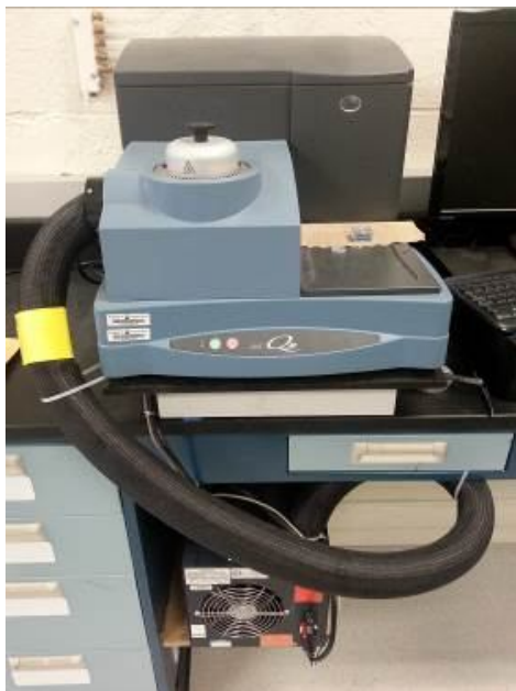
Figure 19: Q20 TA Instrument DSC system
