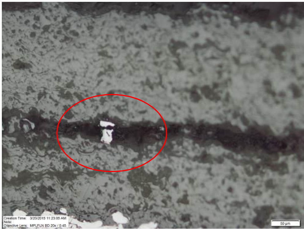
Figure 47: Microstructure of pullout in crack along the coating at 20x magnification
