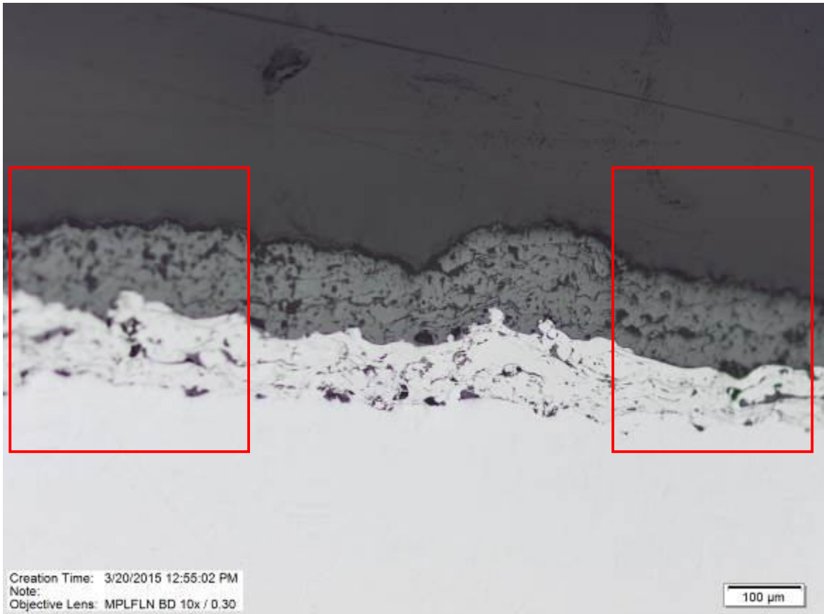
Figure 35: Microstructure of 10 °C/min to 55 °C with uneven surface
