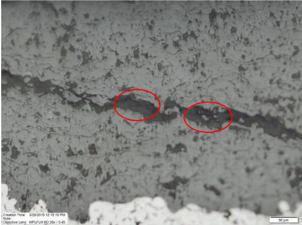
Figure 33: Microstructure of 5 °C/min to 55 °C under 20x magnification of crack
