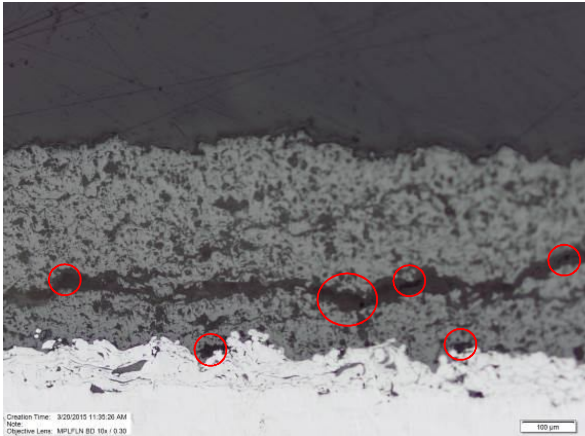
Figure 40: Microstructure of epoxy heated prior to mounting at 5 °C/min to 55 °C
