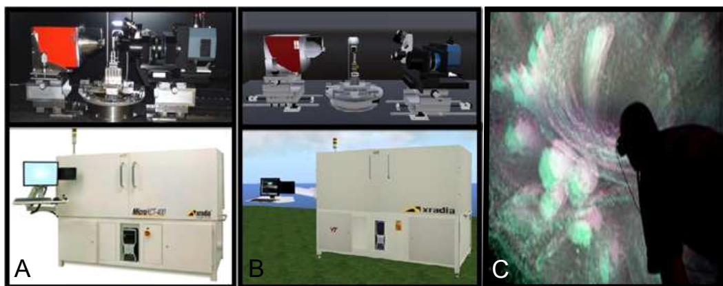
Figure A.2: Training and education, and volume visualization. (A) Xradia MicroXCT-400 scanner (bottom) and internal components (top). (B) Virtual replica in Second Life. (C) A participant experiencing a training data-set in the Viscube at Virginia Tech
