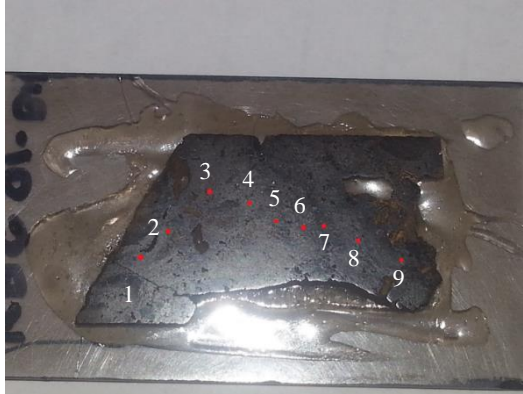
Figure 8: Thick section of RBG01-BH. Numbered red dots represent the sampling points analyzed on the LA-ICPMS.
