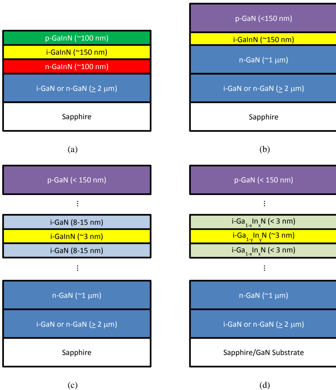
Figure 3.6. Schematic layer structure for contemporary GaInN/GaN solar cells. Upper Left (a): GaInN homojunction. Upper Right (b): GaInN/GaN double heterojunction. Lower Left (c): GaInN/GaN MQW structure. Lower Right (d): GaInN/GaInN superlattice structure.
