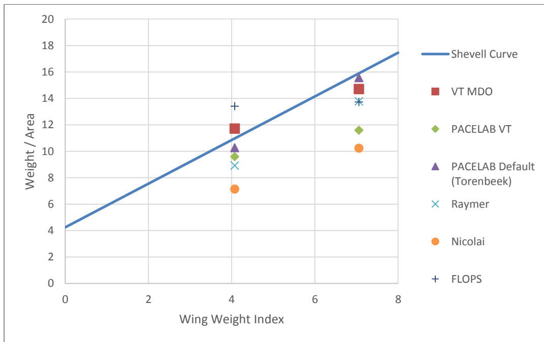
Figure 40. Shevell's wing weight curve with predictions from VT MDO, PACELAB APD 3.1 (Torenbeek), PACELAB-VT (Locatelli), Raymer and Nicolai. 737-800 on the left, 777 on the right.
