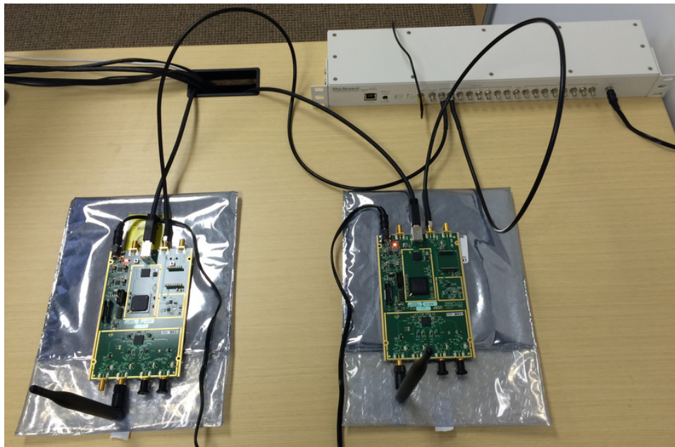
Figure 3.7: The hardware setup for the over-the-air experiment. The transmitter (left) and receiver (right) are both B210 USRPs with Vert900 antennas. An Ettus Octoclock-G is used to minimize the frequency and timing drift experienced during observation periods.
