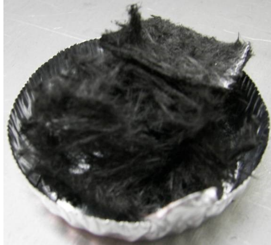
Figure 5-15. Network of carbon fibers after unconstrained pyrolysis.
