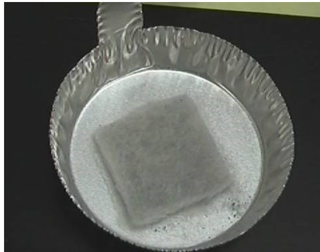
Figure 5-14. Network of glass fibers after fully constrained pyrolysis.
