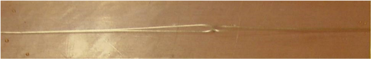
Figure 6.3-5. Fiber form with cured epoxy maintaining the shape.
