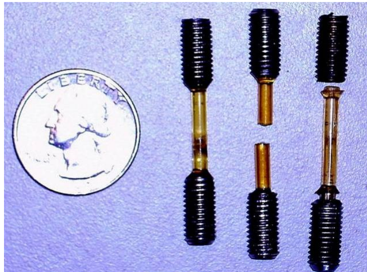
Figure 6.4-9. D2-3 samples (from left to right) untested, failed in gage length, grip failure and pull-out.
