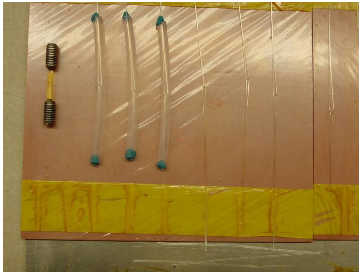
Figure 6.3-6. Fiber form (right) was inserted in Teflon tube and bottom sealed with clay (middle) to produce a specimen (left).
