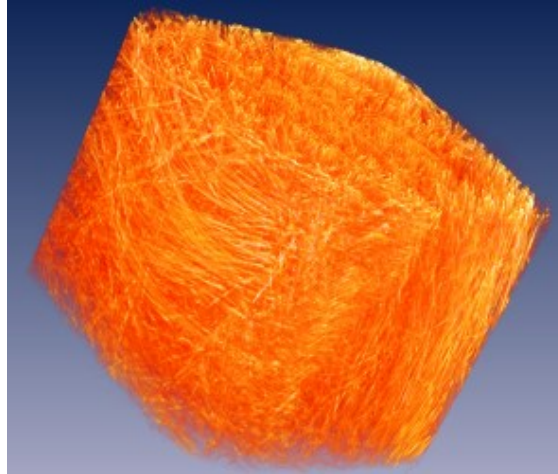
Figure 2-3. X-ray computed tomography reconstruction for injection molded composite.
