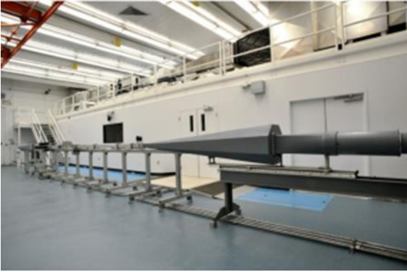
Figure 12. Grazing Flow Impedance Tube (GFIT): (left) Main floor of GFIT with flow from left to right; (right) microphone instrumentation
