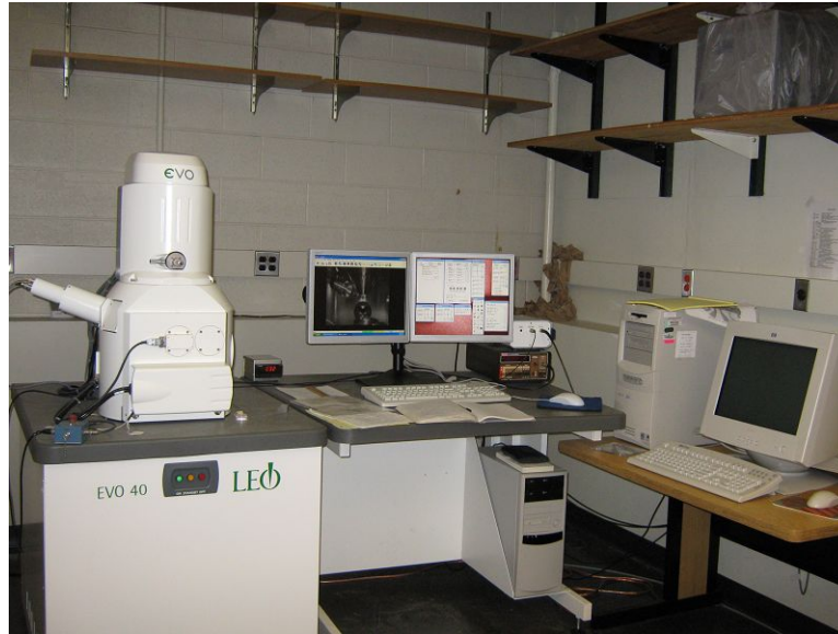
Figure 2.6: E-beam lithography setup, it's an SEM integrated with an electron beam control module.
