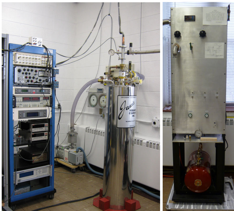
Figure 3.1: Measurement system. In the left photograph, the Janis dewar and associated electronic instruments to supply power and magnetic field, measure the sample and monitor the system are shown. The right photograph shows the ^3\text{He} system (home built).
