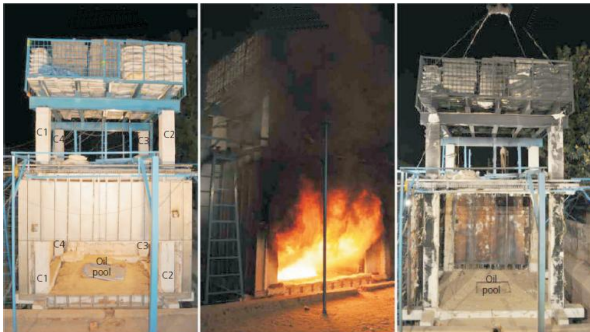
Figure 2.7. Reinforced concrete frame subjected to fire testing after earthquake damage. Bhargava, P., Kamath, P., Usmani, A., May, I., B Singh, B., Gillie, M., Sharma, U. K., Kumar, V., Pankaj, P., Torero, J., Y Singh, Y., and Zhang, J. (2012). “Full-scale testing of a damaged reinforced concrete frame in fire.” Proceedings of the ICE - Structures and Buildings , 165, 335–346. Used under fair use, 2015.
