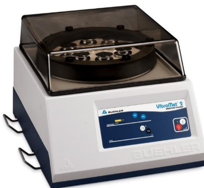
Figure 2.2. Picture of the vibratory polisher used for the eight-hour final polishing step. ( https://shop.buehler.com/equipment/auxiliary-support-equipment/products/vibromet-2-vibratory-polisher ) Used under fair use, 2015.
