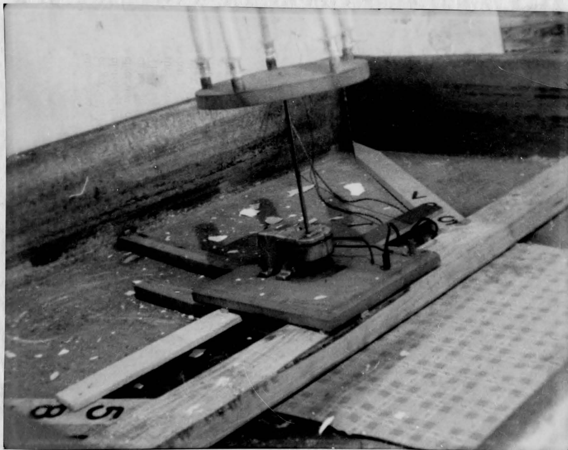
Apparatus for holding and rotating bottles during spraying
