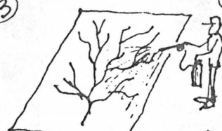
a clear plastic sealant is applied
