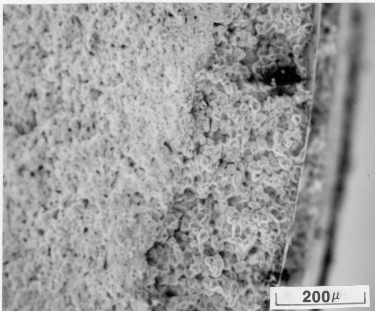
Figure 6. Fractograph of specimen 19 showing crack mode transition. Definition between intergranular, environmentally induced crack and ductile, microvoid rupture.
