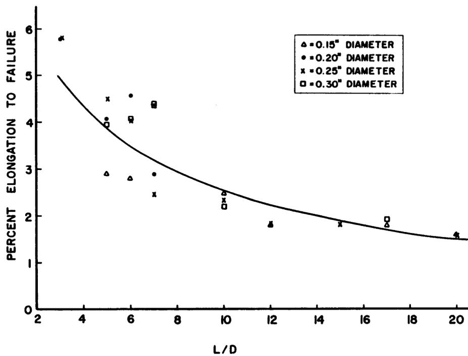
Figure 18. Percent elongation to failure plotted as a function of specimen dimensions. Curve fit using a reciprocal regression.
