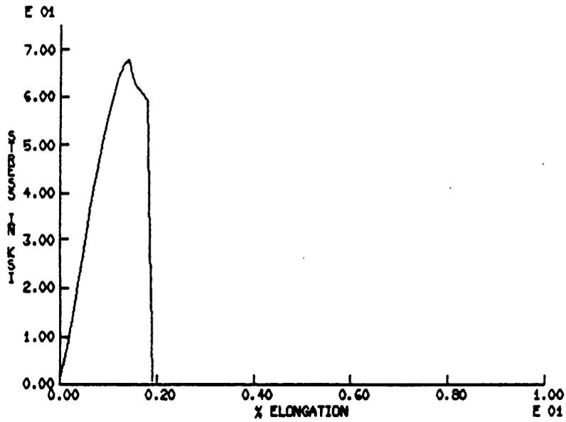
Figure 15. Engineering stress - percent elongation curve for specimen 18 ( $\frac{L}{D} = 17$ ).
