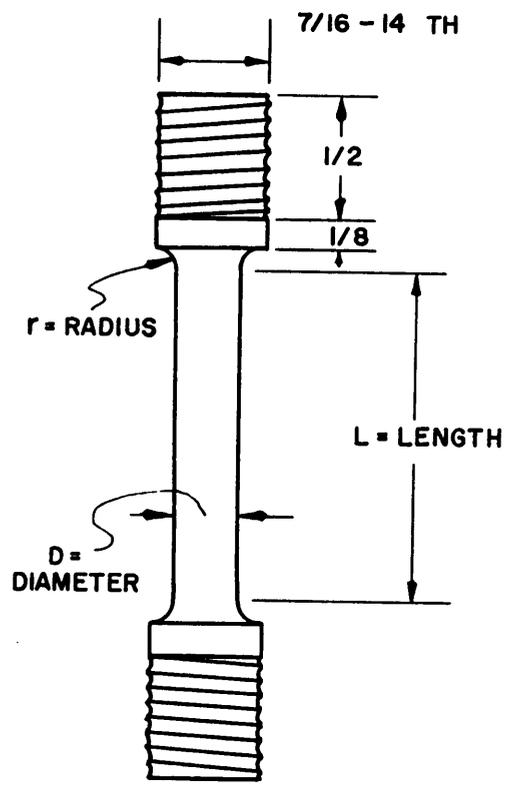
Figure 2. Tensile specimen geometry.
