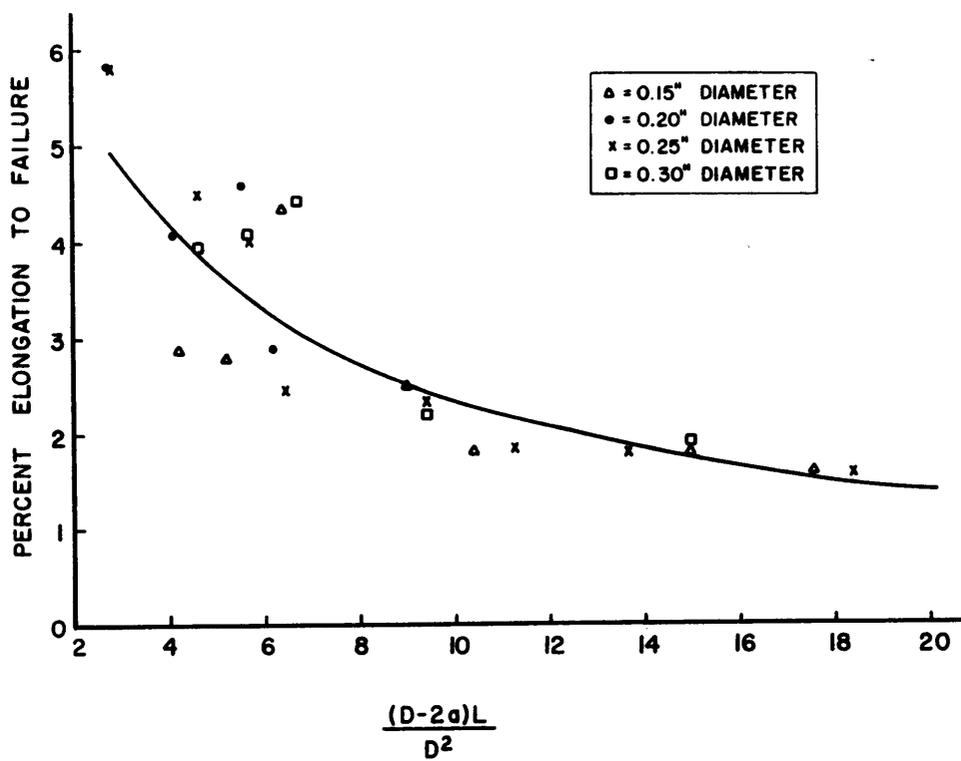
Figure 19. Percent elongation to failure plotted as a function of T applied.
