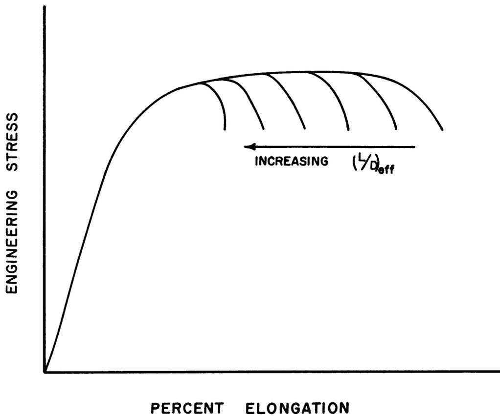
Figure 17. Idealized effect of increasing specimen dimensions. Elongation to failure decreases with increasing  $(\frac{L}{D})_{eff}$
