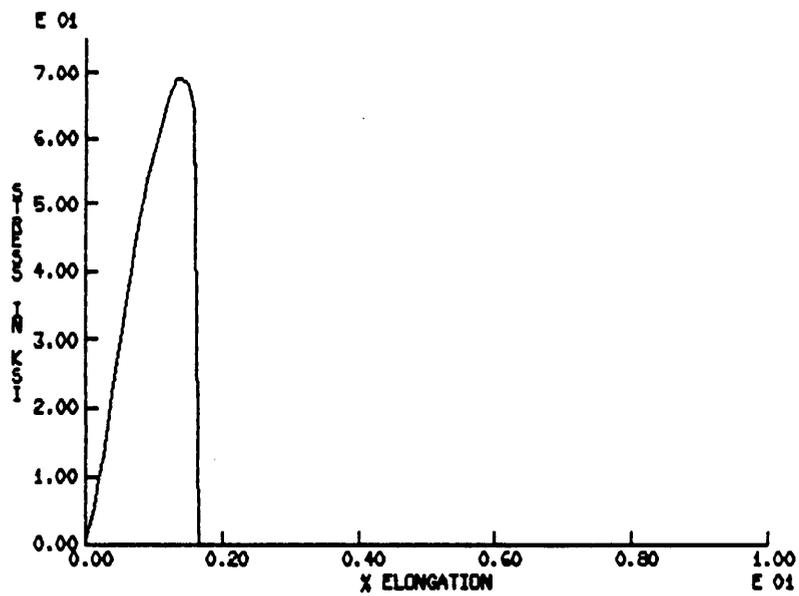
Figure 16. Engineering stress - percent elongation curve for specimen 19 ( $\frac{L}{D} = 20$ ).
