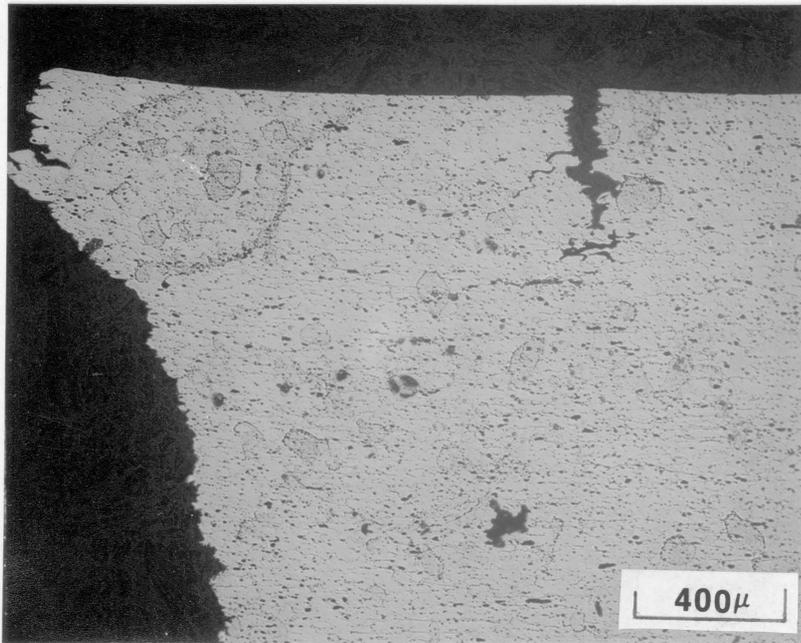
Figure 25. Micrograph of secondary environmental cracking in specimen 43. (D = 0.30 inch).
