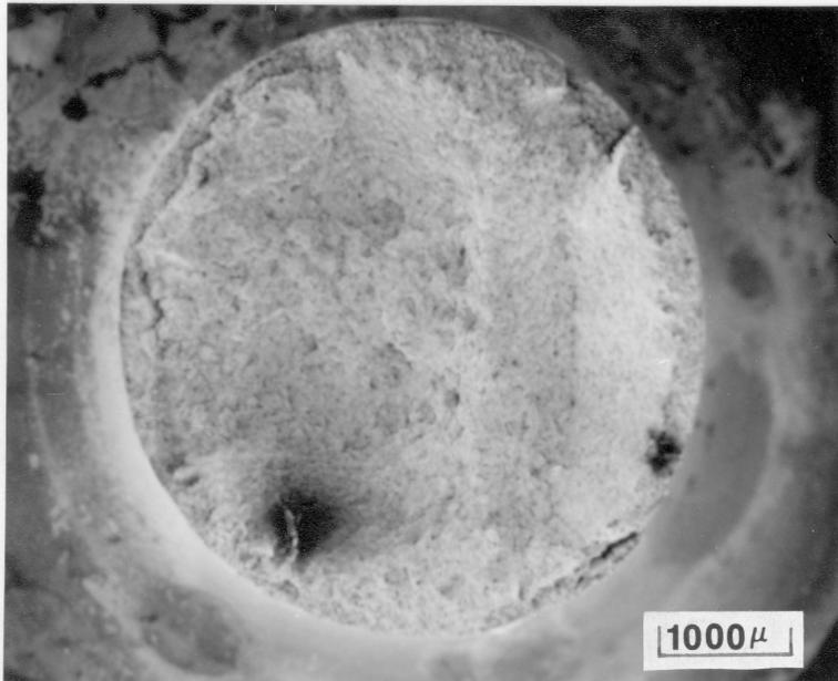
Figure 5. Fractograph of specimen 19 showing annular crack.
