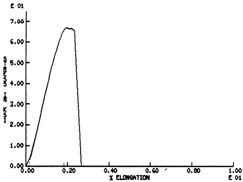
Figure 12. Engineering stress - percent elongation curve for specimen 45 ( $\frac{L}{D} = 10$ ).
