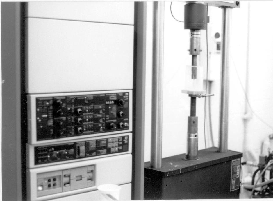
Figure 3. Experimental set-up with MTS model 810 Materials Test System and environmental containment vessel.
