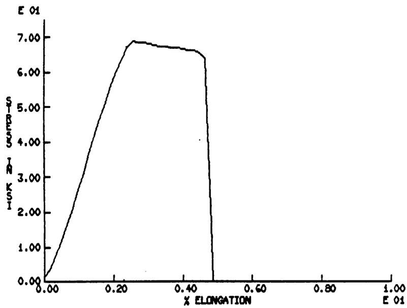
Figure 9. Engineering stress - percent elongation curve for specimen 32 ( $\frac{L}{D} = 5$ ).
