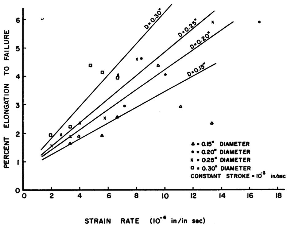
Figure 21. Percent elongation to failure as a function of strain-rate. The four different lines represent linear regressions of the data of the four different diameter sizes.
