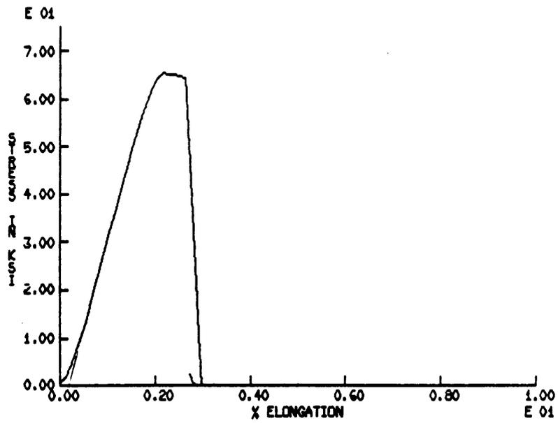
Figure 11. Engineering stress - percent elongation curve for specimen 34 ( $\frac{L}{D} = 7$ ).
