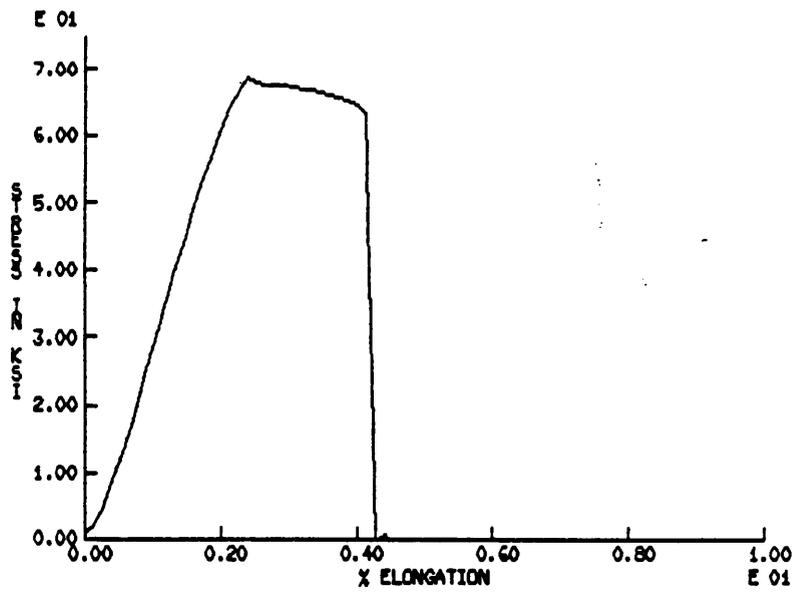
Figure 10. Engineering stress - percent elongation curve for specimen 33 ( $\frac{L}{D} = 6$ ).
