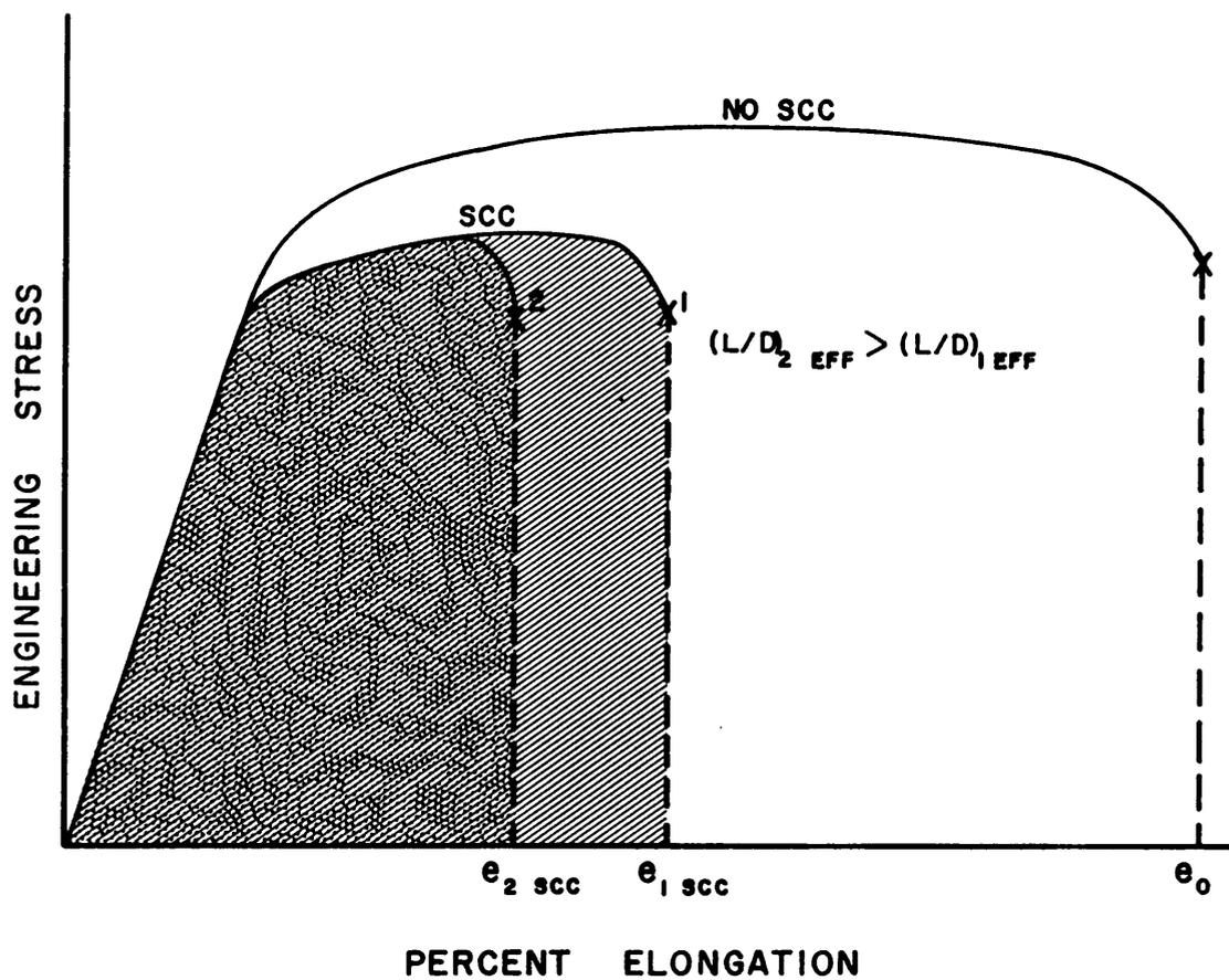
Figure 20. Effect of specimen dimensions on SCC evaluation. Engineering stress - elongation curve illustrating the possible effect of differences in specimen dimensions on measured SCC evaluation parameters.
