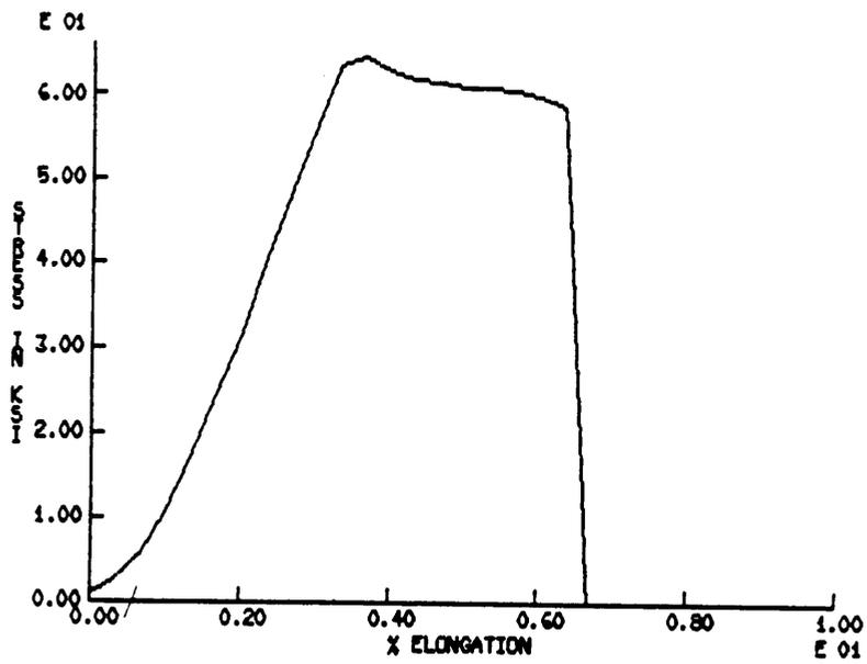
Figure 8. Engineering stress - percent elongation curve for specimen 21 ( $\frac{L}{D} = 3$ ).
