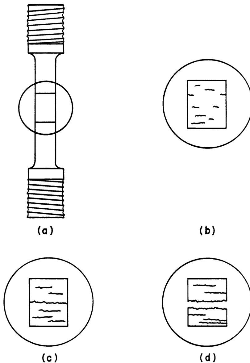
**Figure 4.** Schematic of expected crack growth chronology in fracture process. (a) Specimen at start of test (b) enlarged view of exposed region of specimen with cracks beginning to grow perpendicular to axis of loading as test proceeds, (c) with increasing time and strain, crack grows radially, (d) finally, a crack will become annular and final fracture occurs on the plane of this crack, perpendicular to axis of loading.
