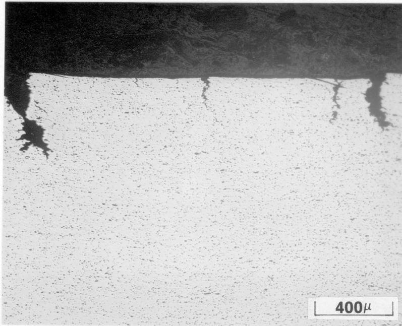
Figure 24. Micrograph of secondary environmental cracking in specimen 13. (D = 0.15 inch).
