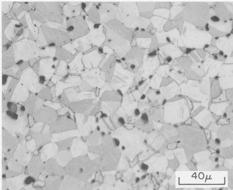
**Figure 1. Microstructure of Free Machining Brass.**
