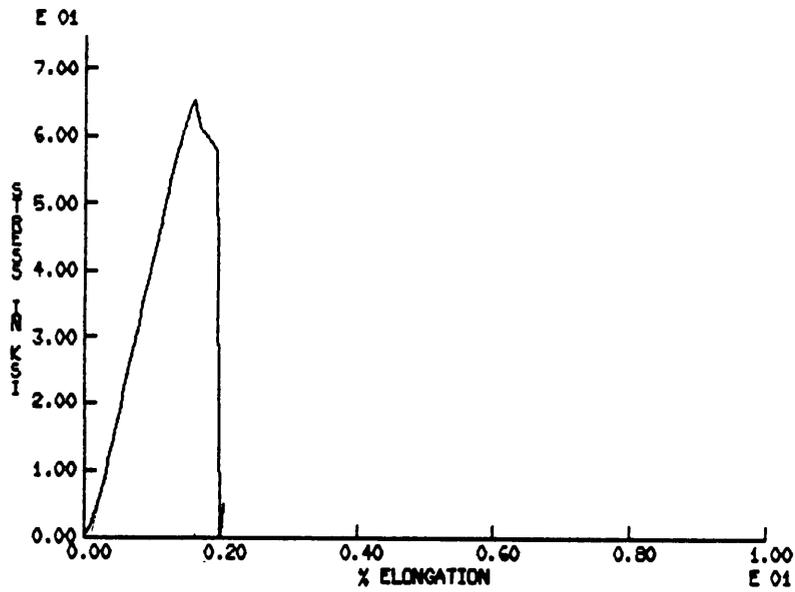
Figure 14. Engineering stress - percent elongation curve for specimen 37 ( $\frac{L}{D} = 15$ ).
