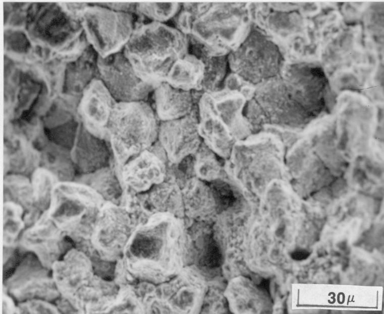
Figure 7. Fractograph of specimen 19 showing intergranular crack. Nature of the environmentally induced crack.
