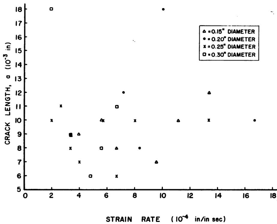
Figure 22. Plot of crack length as a function of strain-rate.
