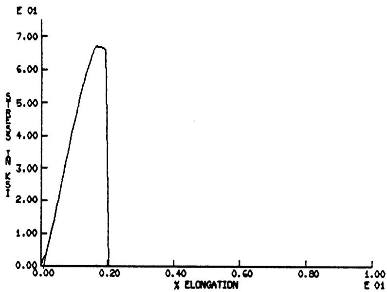
Figure 13. Engineering stress - percent elongation curve for specimen 36 ( $\frac{L}{D} = 12$ ).
