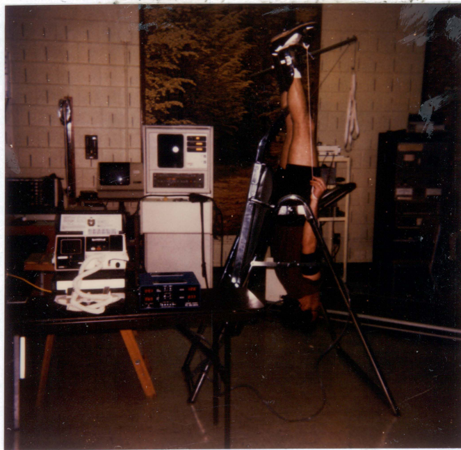
Figure 3. Photographs of subjects in the standing and inverted posture on the gravity oscillator.
