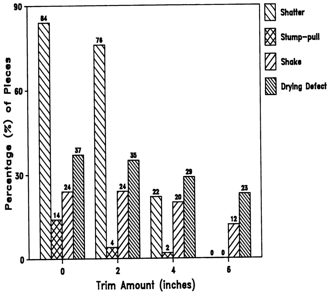
Figure 8. Percentage of pieces with indicated defects per trim class for the Large Acceptable Log Class (Federal Paperboard Co.).
