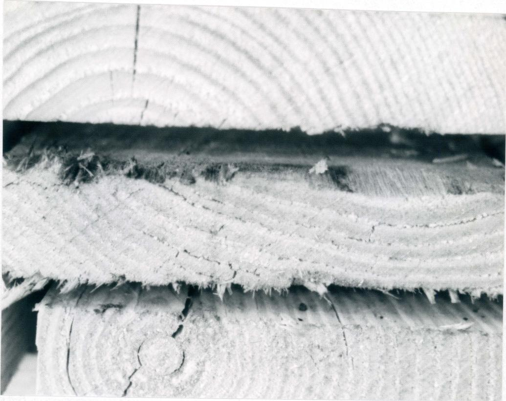
Figure 3. Lumber end showing shatter damage (middle piece).
