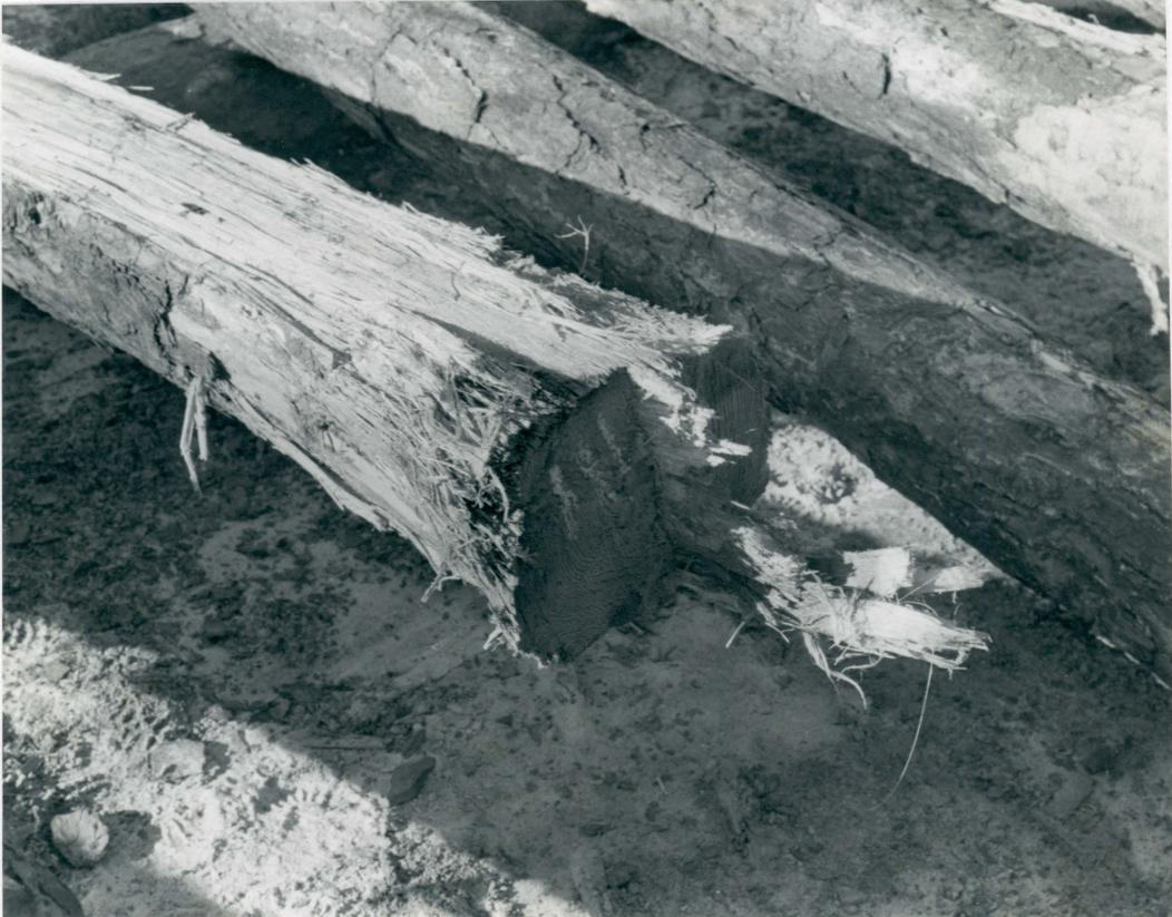
Figure 2. Unacceptable log showing stump-pull extending from the butt.
