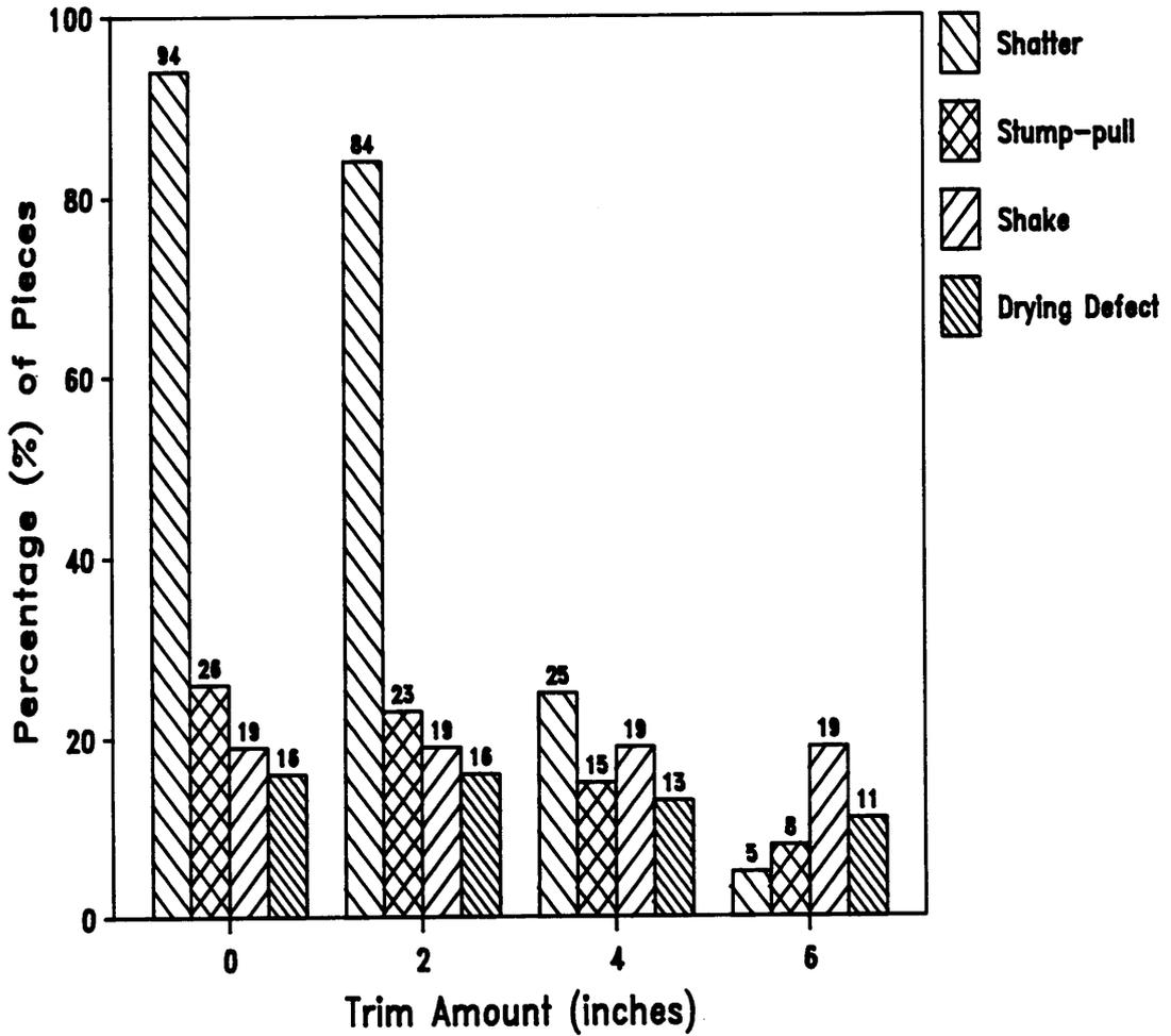
Figure 9. Percentage of pieces with indicated defects per trim class for the Large Unacceptable Log Class (Federal Paperboard Co.).
