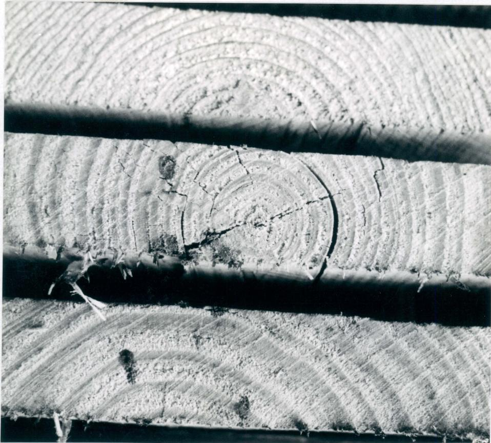
Figure 4. Lumber end showing ring shake.
