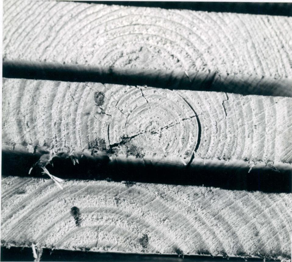
Figure 4. Lumber end showing ring shake.
