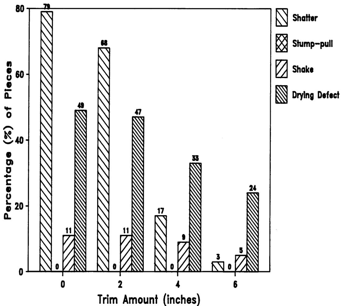
Figure 6. Percentage of pieces with indicated defects per trim class for the Small Acceptable Log Class (Federal Paperboard Co.).
