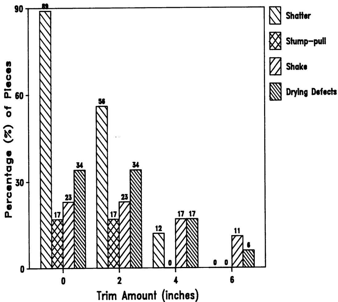
Figure 12. Percentage of pieces with indicated defects per trim class for the Small Unacceptable Log Class (Bowater Lumber Co.).
