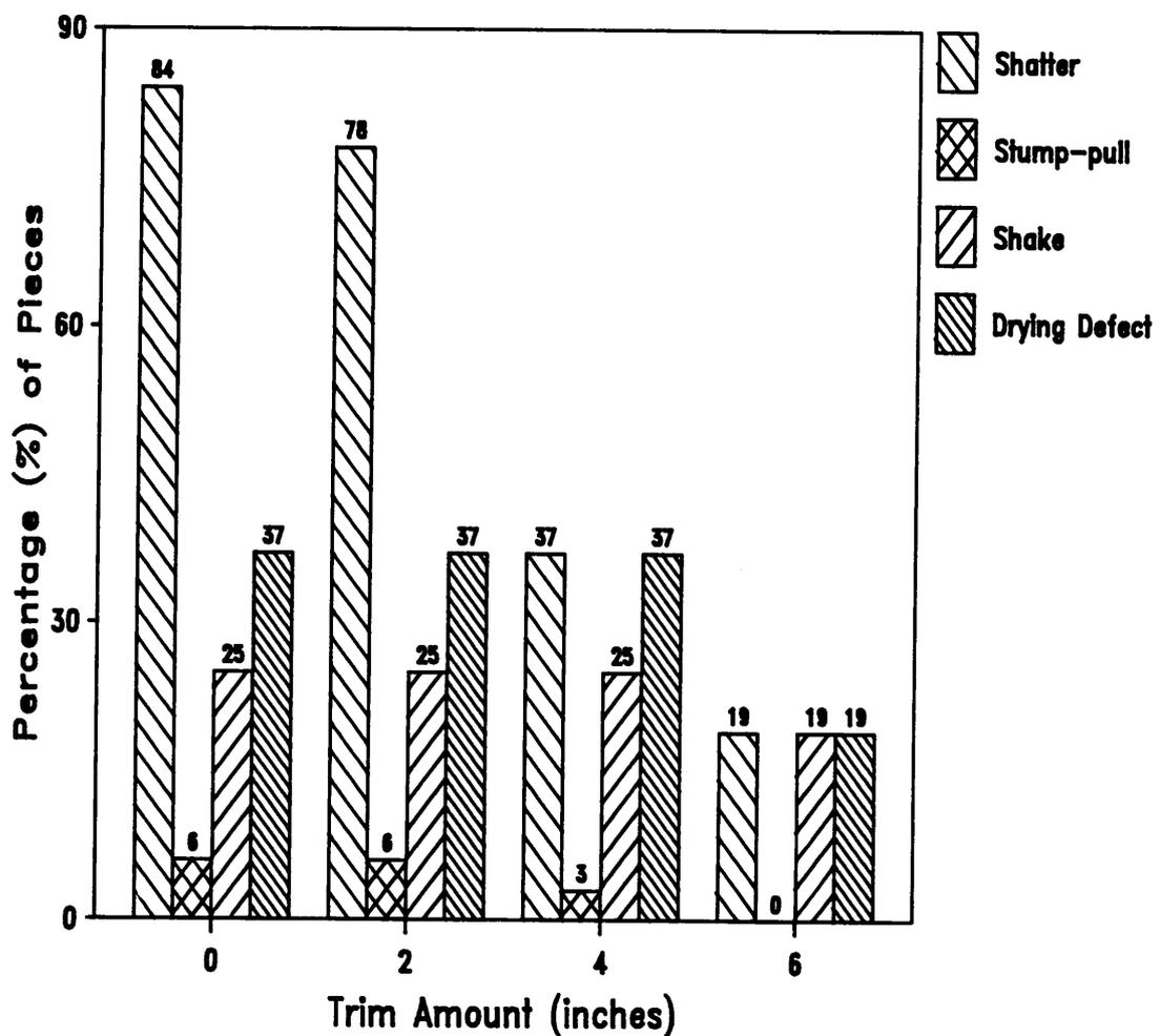
Figure 7. Percentage of pieces with indicated defects per trim class for the Small Unacceptable Log Class (Federal Paperboard Co.).
