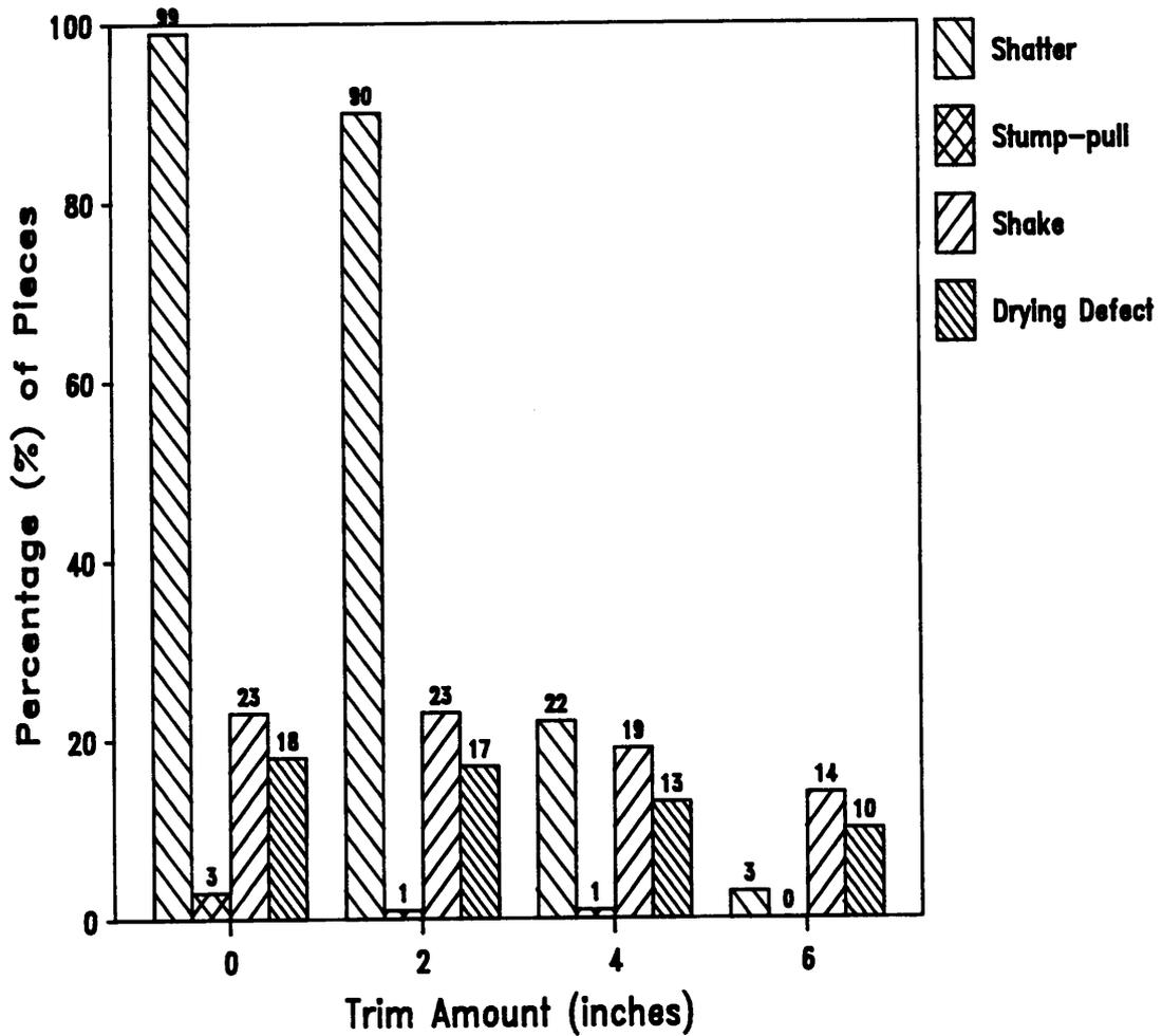
Figure 13. Percentage of pieces with indicated defects per trim class for the Large Acceptable Log Class (Bowater Lumber Co.).
