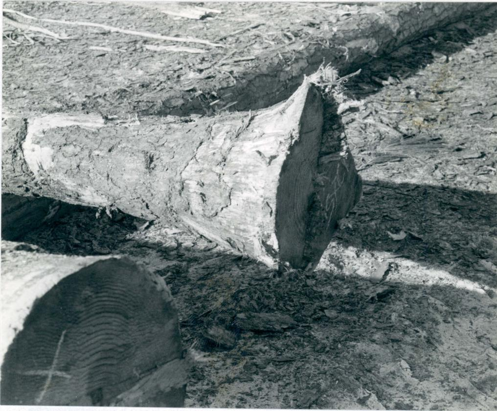
Figure 1. Log showing butt flare or swell.
