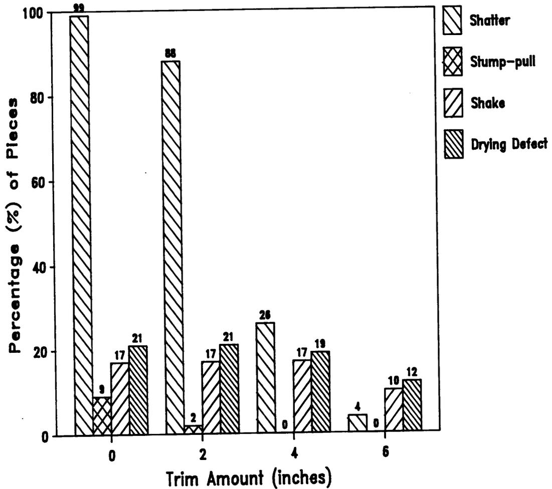
Figure 11. Percentage of pieces with indicated defects per trim class for the Small Acceptable Log Class (Bowater Lumber Co.).
