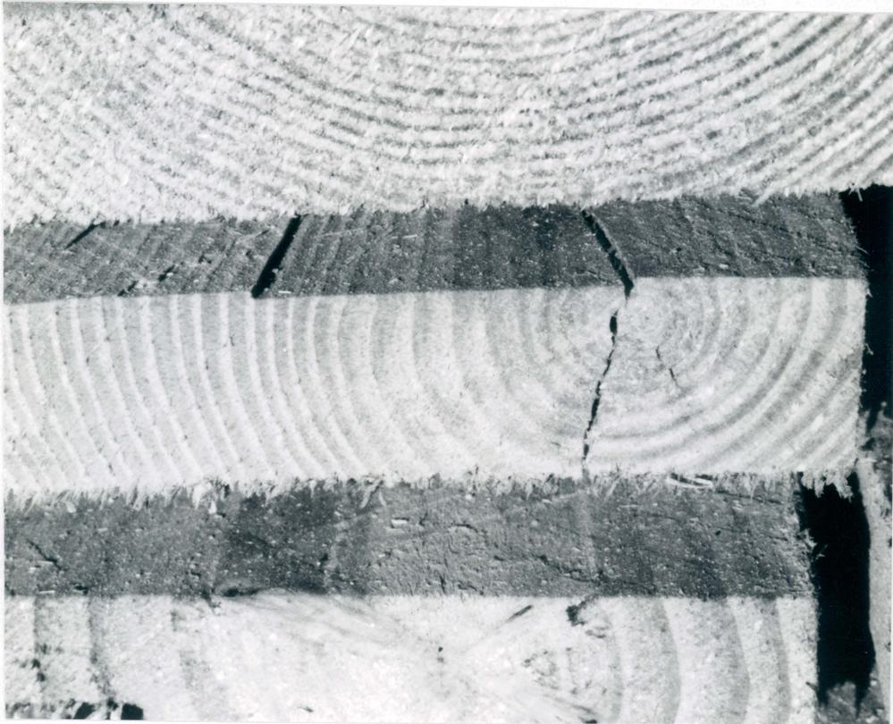
Figure 5. Lumber end showing drying split.
