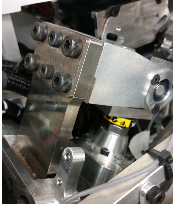
Figure 2.16: Actuator attachment to the configurable compliant spring.
