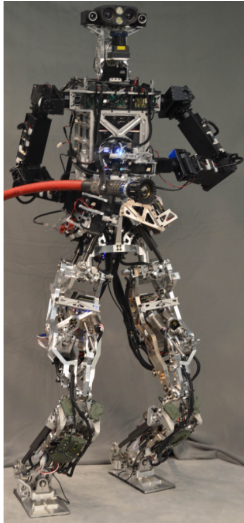
Figure 1.3: Tactical Hazardous Operations Robot (THOR), photographed by and used with permission of Eric Hahn, 2014.
