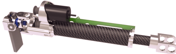
Figure 1.2: Rendering of the linear SEA used on SAFFiR, from “Design and Measurement Error Analysis of a Low-Friction Lightweight Linear SEA,” used with permission of Bryce Lee, 2014.
