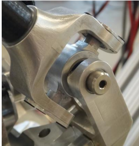
Figure 2.15: Lower universal joint for the ankle actuators.
