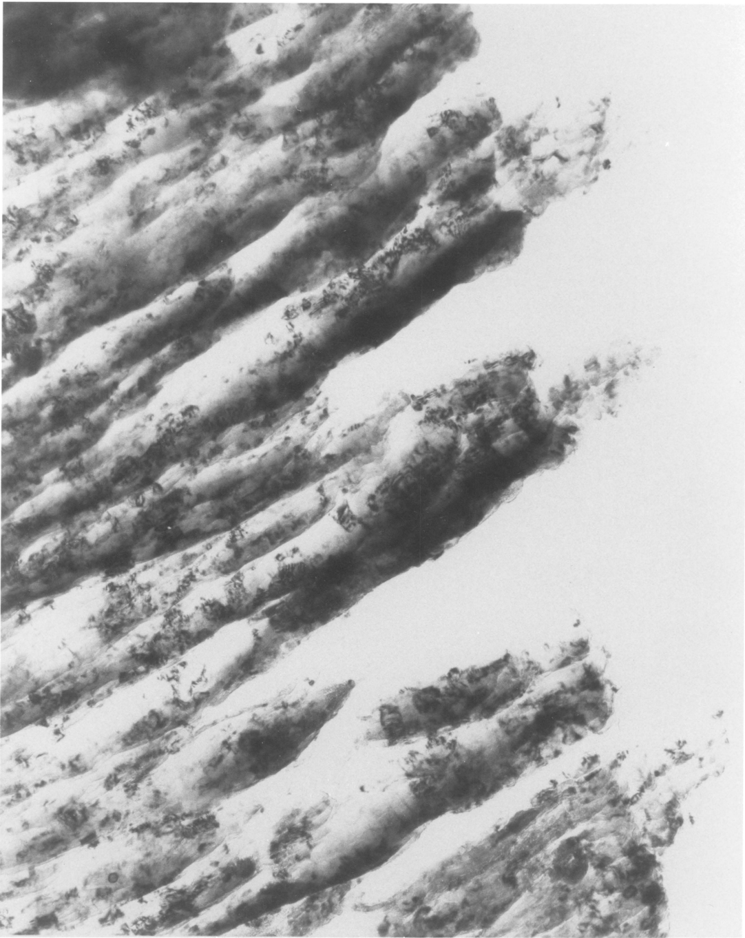
Figure 28. Transmission electron micrograph of ultramicrotomed section cut transversely through PAA Al/Li oxide-polysulfone interface, 29,000 X.
