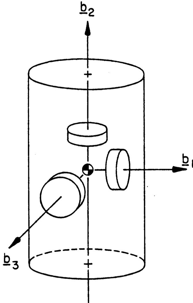
Figure 5.1 Rigid Spacecraft with Three Orthogonal Reaction Wheels
