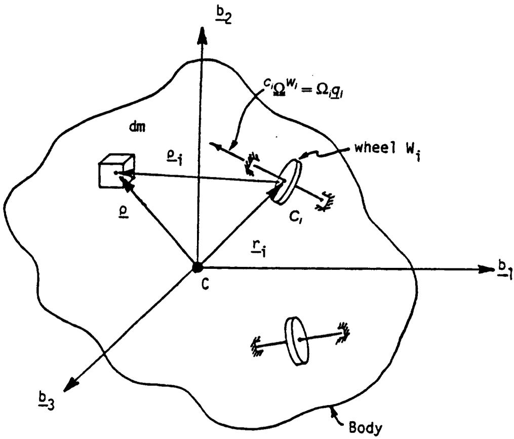
Figure 3.1 Rigid Spacecraft with N Reaction Wheels
