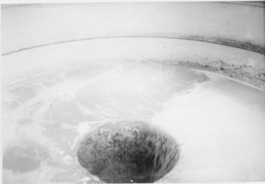
Figure 8: Pump Induced Foam During Phase 1 Experiments The photograph illustrates the appearance of pump induced foam at maximum recirculation rate (43 gpm.) and zero aeration during Phase 1 experiments.
