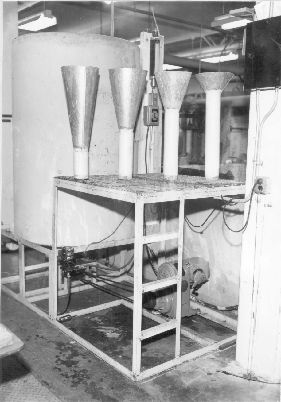
Figure 4: Phase 3 Experimental Unit and Inlet Structures The inlet structures have a top diameter of 12 inches and have depths of 24, 18, 12, and 6 inches respectively from left to right.
