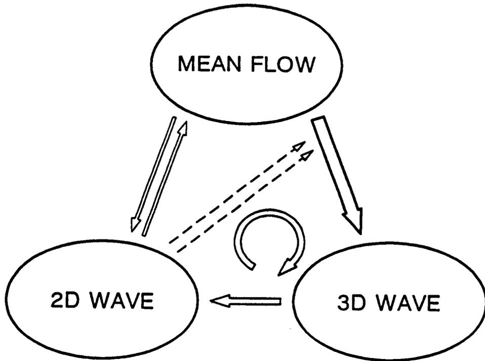
Figure 1.1 Schematic of energy transfer between the mean flow and the two- and three-dimensional waves. The dashed line signifies a catalytic effect. Taken from Herbert (1988a).
