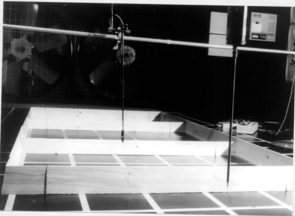
Figure 34 Photograph of wind tunnel floor, full citadel model with internal walls, wind from the south. Upwind reference Probe 1 is in the foreground and data Probe 4 is inside the model in the background.
