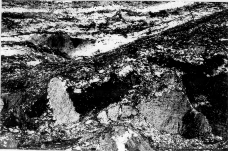
Fig. 40. Mylonite of Little River Gneiss showing elongate quartz ribbons with deformation bands parallel to S and recrystallization along deformation band m boundaries, note thinning and deflection around augen pod; 1 cm = .18 mm, sample #B-11.
