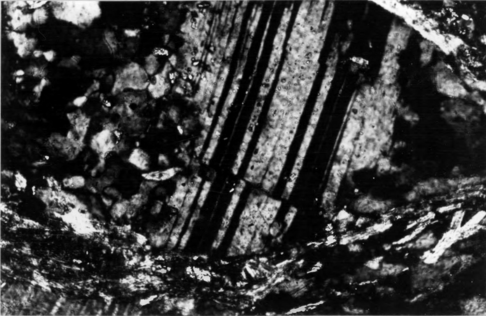
Fig. 52. Offset twin planes along microfracture in plagioclase (Little River Gneiss); 1 cm = .04 mm, sample #44 (see appendix).
