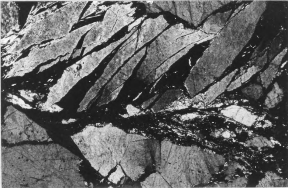
Fig. 77. Relatively undeformed and unaltered coarse grained amphibolite showing large hornblende crystals with minor alteration to chlorite (dark areas between grains); 1 cm = .28 mm, sample #247 (see appendix).
