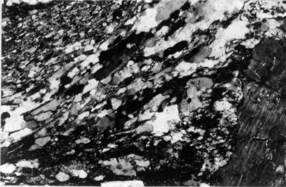
Fig. 42. Quartzose stringers thinned around augen in mylonite of Little River Gneiss with subgrains and recrystallized grains have a shape preferred orientation parallel to S ; 1 cm = .12 mm, sample #I-5 m (see appendix)
