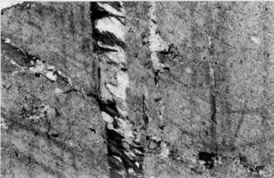
Fig. 50. Quartz fiber growth along fracture in alkali feldspar augen, dark areas are biotite; 1 cm = .1 mm, sample #B-18 (see appendix).
