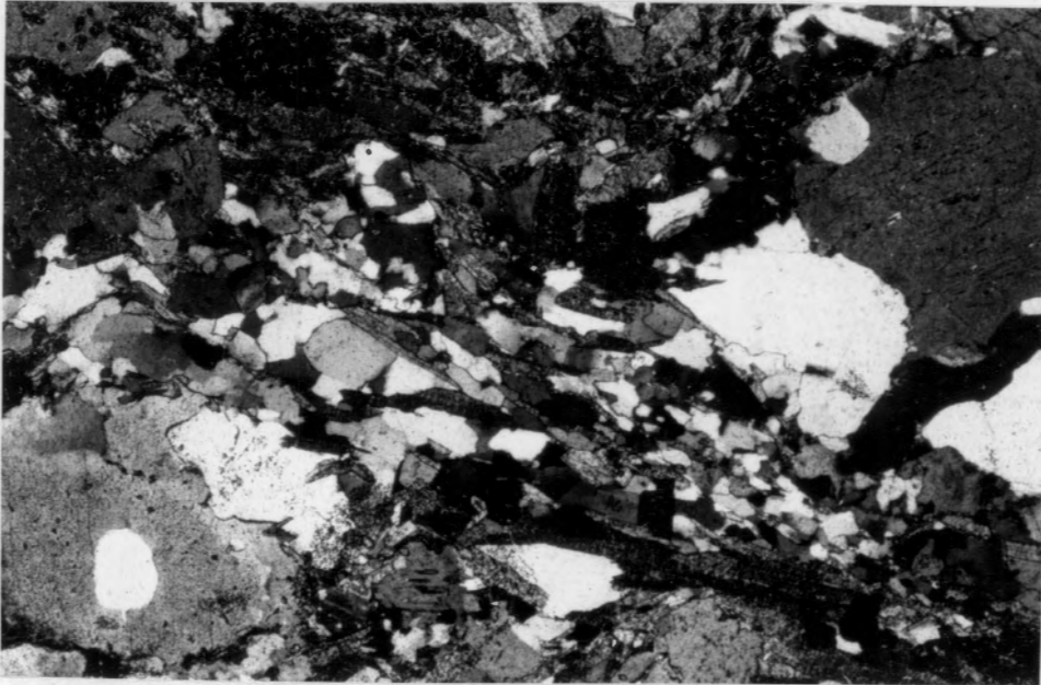
Fig. 32. Thin section of non-mylonitized Little River Gneiss showing close up of matrix; S_1 foliation defined by large biotites and muscovites; 1 cm = .29 mm, sample #296 (see appendix).
