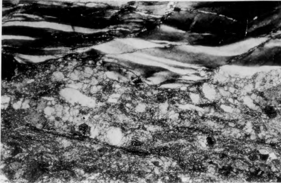
Fig. 59: Pilot Gneiss mylonite in which S_m is defined by elongate quartzose ribbons alternating with quartzo-feldspathic rich zones. 1 cm = .27 mm, sample #E-1(4a) (see appendix).
