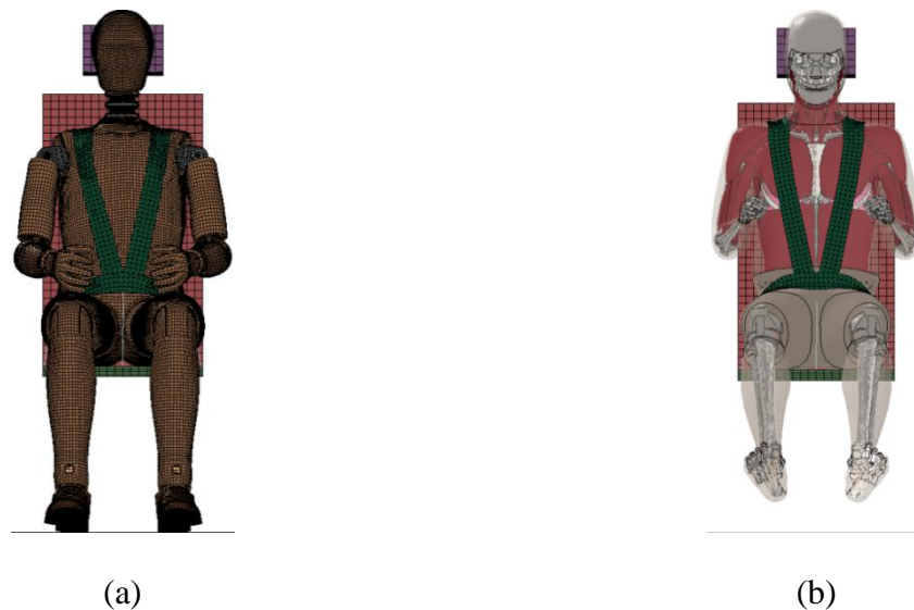
Figure 6-6: Front view of a generic five-point restraint system for the (a) ATD_{exp} and (b) GHBMC simulations at t=0 ms. The lap belt and shoulder harness were modeled as a combination of shell and seat belt elements, while the center lap belt tiedown was modeled solely as seatbelt elements.
