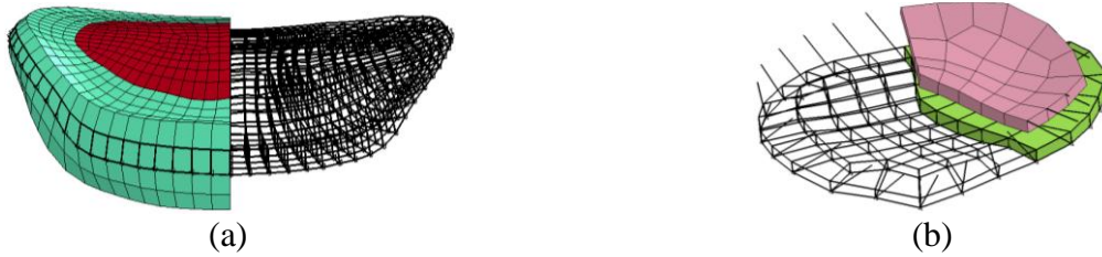
Figure 5-3: Representative cross section set used to capture the load transmission through the (a) IVDs and (b) solid cartilage and beam ligaments of the facets.
