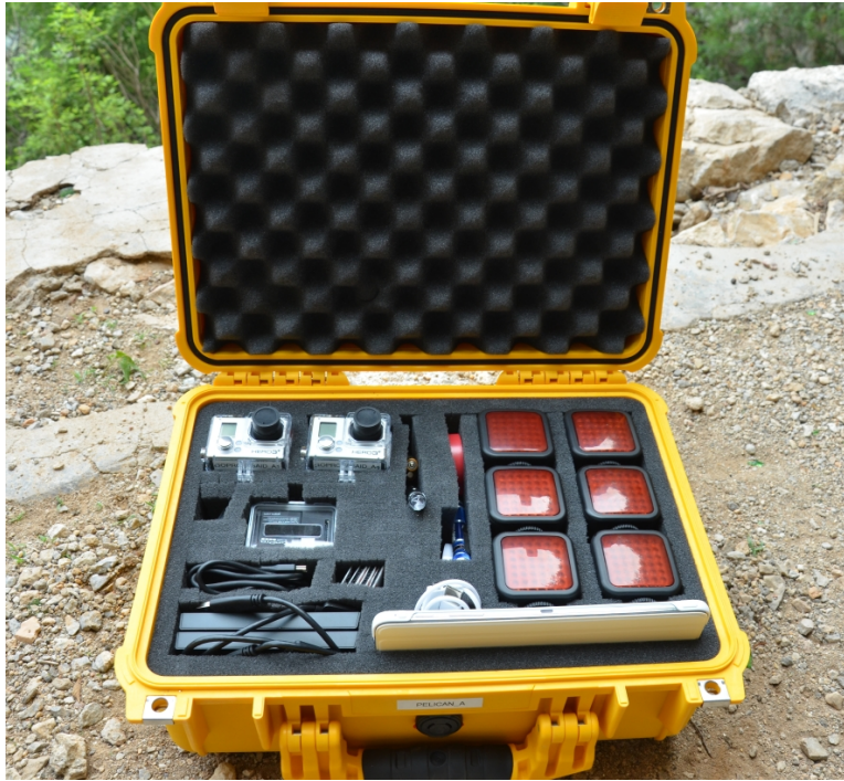
Figure 1.3: All camera system components fit into a 42cm \times 33.1cm \times 17.4cm pelican case for transport.
