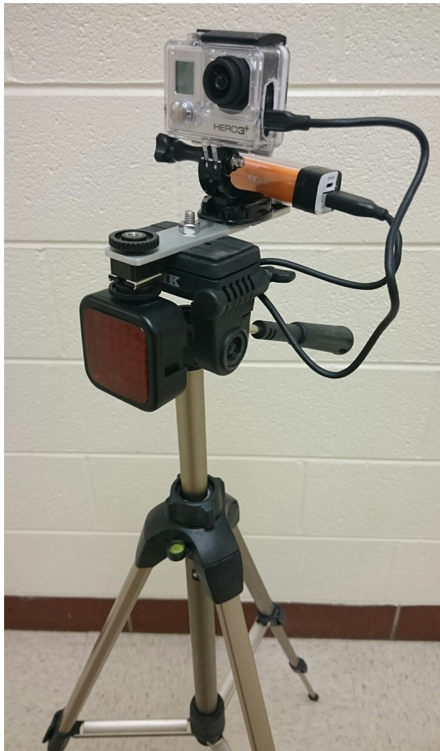
Figure 1.2: A fully constructed tripod includes one modified GoPro camera, one illuminator, and one external battery.
