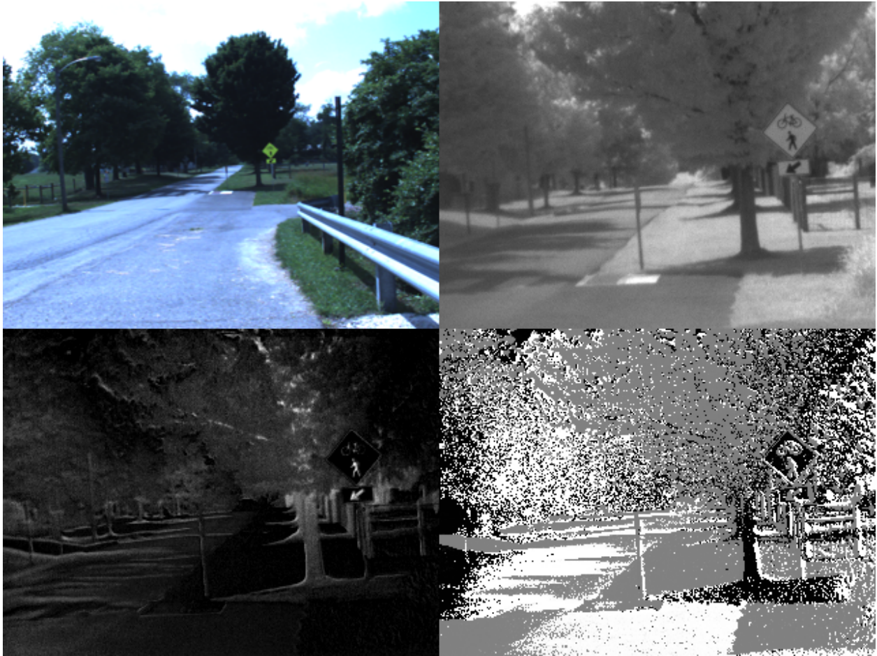
Figure 2.1.10: DoLP and phase for a suburban scene. Clockwise starting at top left: VIS , VIS + NIR I_0 polarization, phase remapped 0-180° to 0-255, DoLP remapped 0-1 to 0-255.
