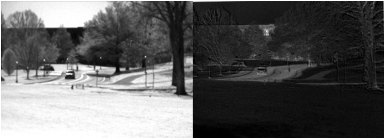
Figure 1.3.6: Example data showing polarization by reflection. Primary targets are asphalt, a building, and a vehicle. Left, image from a horizontal polarized filter. Right, the polarization contrast between horizontal and vertical polarized images[6]. M. Umansky, A. L. Wicks, K. Meehan, and D. W. Hong, "A Prototype Polarimetric Camera for Unmanned Ground Vehicles; Thesis submitted to the faculty of the VPI&SU in partial fulfillment of the requirements for the degree of Master of Science in Mechanical Engineering," Virginia Polytechnic Institute and State University, Tech. Rep., 2013. Used with permission of Mark Umansky, 2015.
