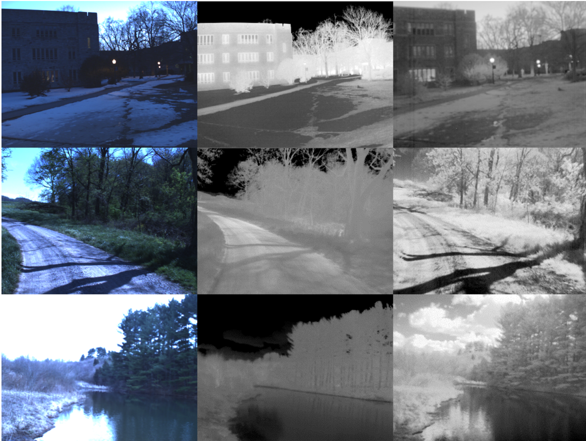
Figure 2.1.5: Examples of low intensity targets in the LWIR band, captured from a Xenics GOBI2689 ( 8 - 14\mu\text{m} ) [10] from the Mechatronics Lab. Left to right: VIS, LWIR, SWIR. Top to bottom: snow, shadow, water.
