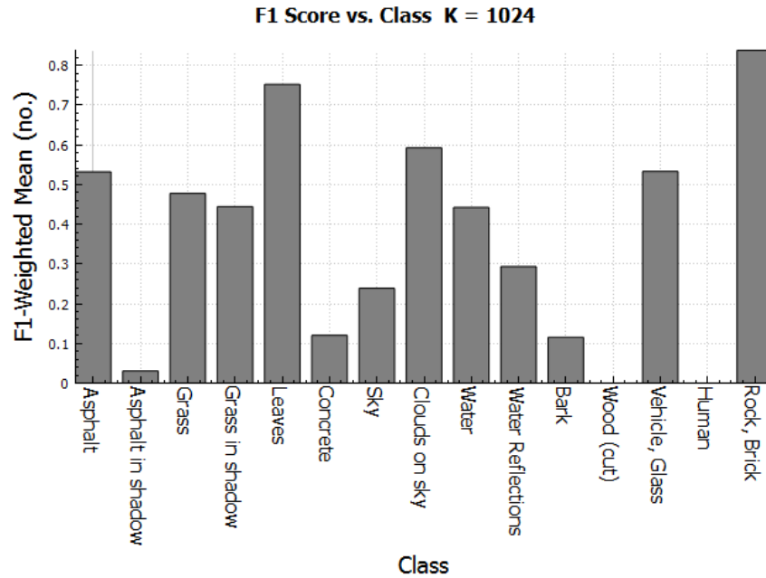
Figure 6.2.4: F1 score vs class index for the K convergence, K = 1024 .
