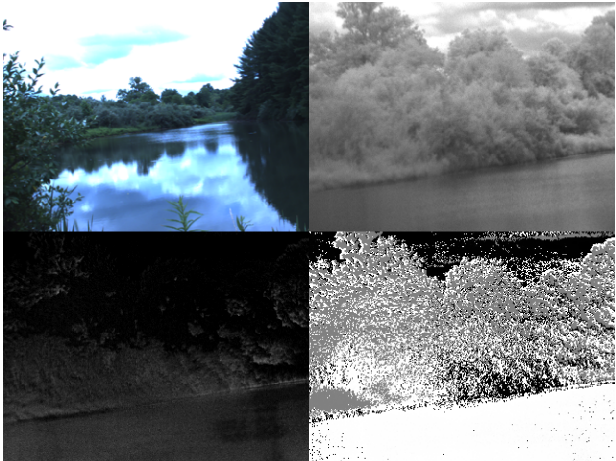
Figure 2.1.12: Example of water reflections in post processed imagery. Clockwise from top left: VIS, Horizontal POLAR, phase remapped from 0 - 180^\circ to 0 - 255 , DoLP remapped from 0 - 1 to 0 - 255 .
