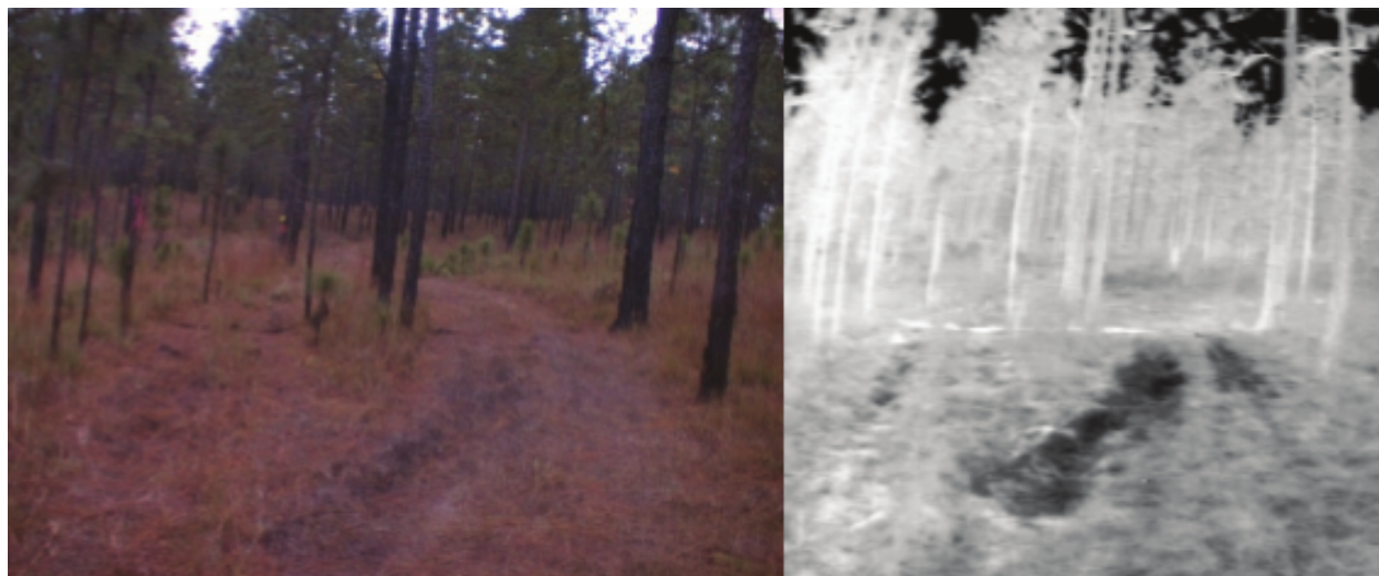
Figure 2.1.6: Example of mud occluded by pine needles, identifiable in the MWIR image (right)[9]. L. H., R. Arturo L, and Matthies, "PASSIVE SENSOR EVALUATION FOR UNMANNED GROUND VEHICLE MUD DETECTION," Jet Propulsion Laboratory, California Institute of Technology, Pasadena, CA, Tech. Rep., 2009. Used under fair use, 2015.
