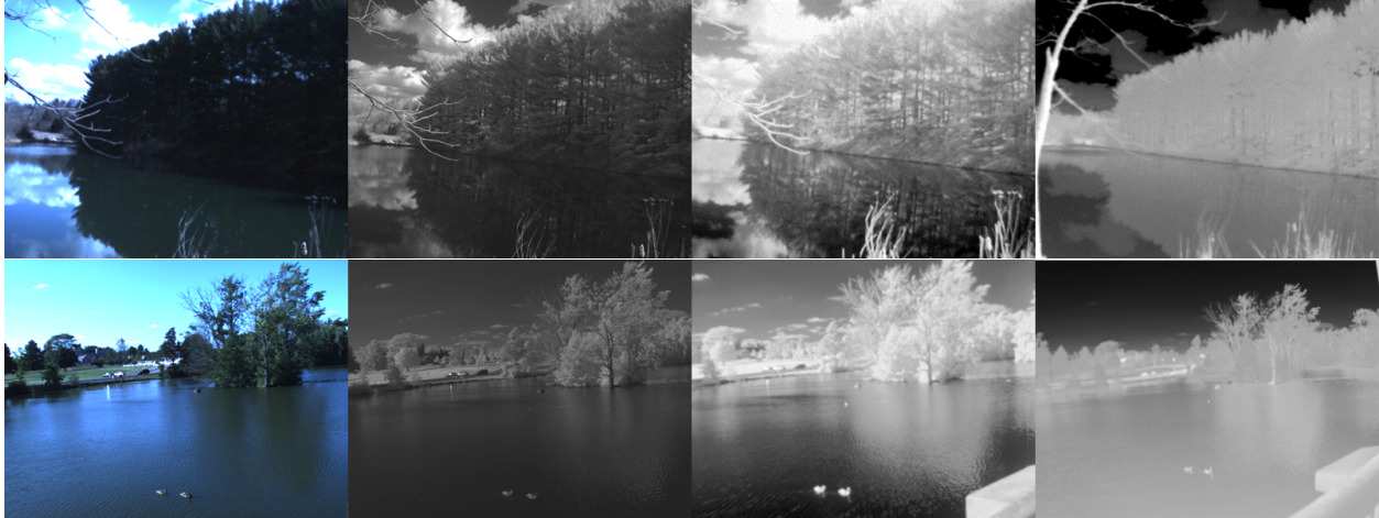
Figure 2.1.11: Examples of reflections off water in raw imagery. Left to right: VIS , NIR , SWIR , LWIR . Note that reflections of cloud, clear sky, and the vegetation is present in all bands. Texture is lost where the water surface is disturbed, seen in the bottom frame.
