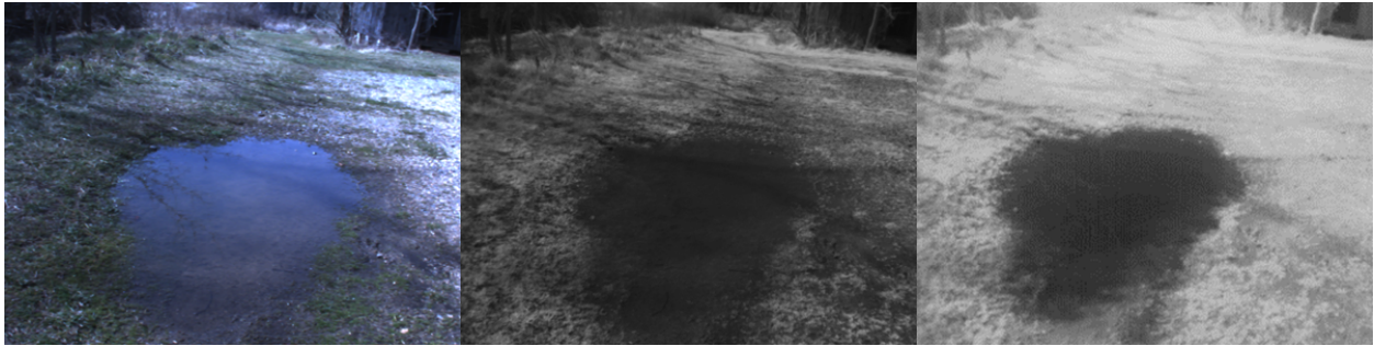
Figure 2.1.15: Example of shallow still water in raw imagery. From left to right VIS , NIR , SWIR .
