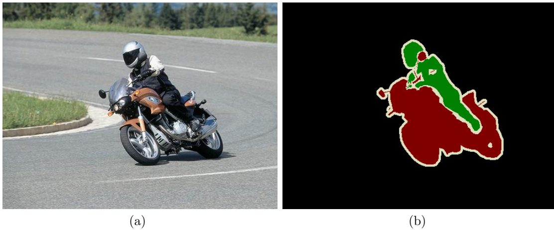
Figure 1.3.7: Example image segmentation. The segmentation is hand labeled, or painted, showing the object classes of human, motorcycle, and void for the object boundaries[45]. M. Everingham, L. Van Gool, C. Williams, J. Winn, and A. Zisserman, "The PASCAL Visual Object Classes Challenge 2012 (VOC2012) Results." [Online]. Available: http://www.pascal-network.org/challenges/VOC/voc2012/workshop/index.html . Used under fair use, 2015.
