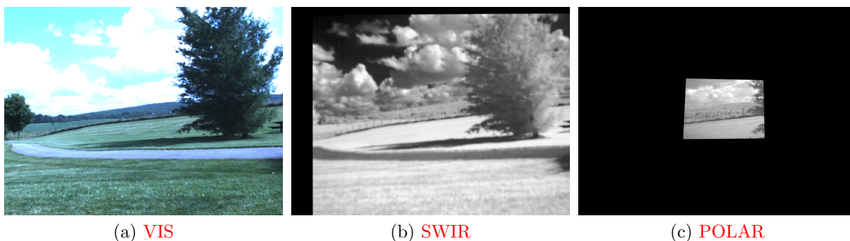
Figure 7.5.1: Example registration illustrating the FoV limitations. Registered images are provided for SWIR and POLAR. The black borders represent the area where the FoV does not overlap.
