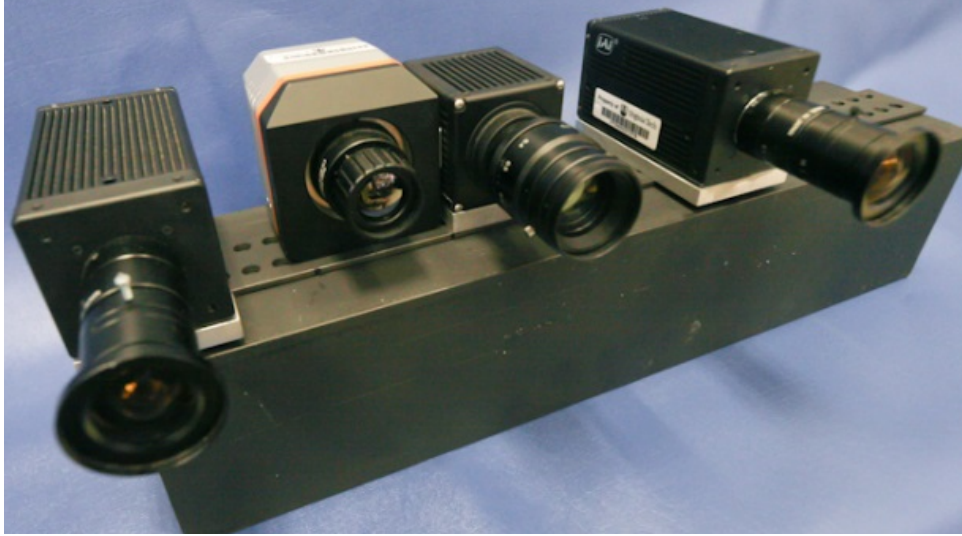
Figure 1.3.1: The multispectral rig used by the Mechatronics Lab at Virginia Tech. From left to right: JAI AD-080GE(VIS/NIR 0.4\mu m - 0.65\mu m , 0.76\mu m - 1.0\mu m )[22], Gobi-384(LWIR: 8\mu m - 14\mu m )[10], SU320HX-1.7RT(SWIR: 0.9\mu m - 1.7\mu m )[23], a second JAI AD-080GE, Polarimetric VIS/NIR camera (not shown) created by the Mechatronics Lab[6] using 4 Point Grey FMVU-03MTM/C(VIS/NIR 0.42\mu m - 1.0\mu m )[24].
