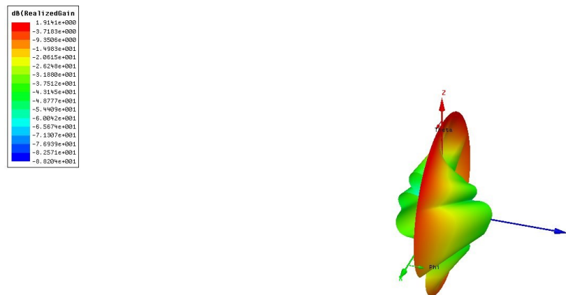
Figure 5.20: 3D Gain pattern of Circular Monopole over 3-Layer EBG Structure at 0.8 GHz.
