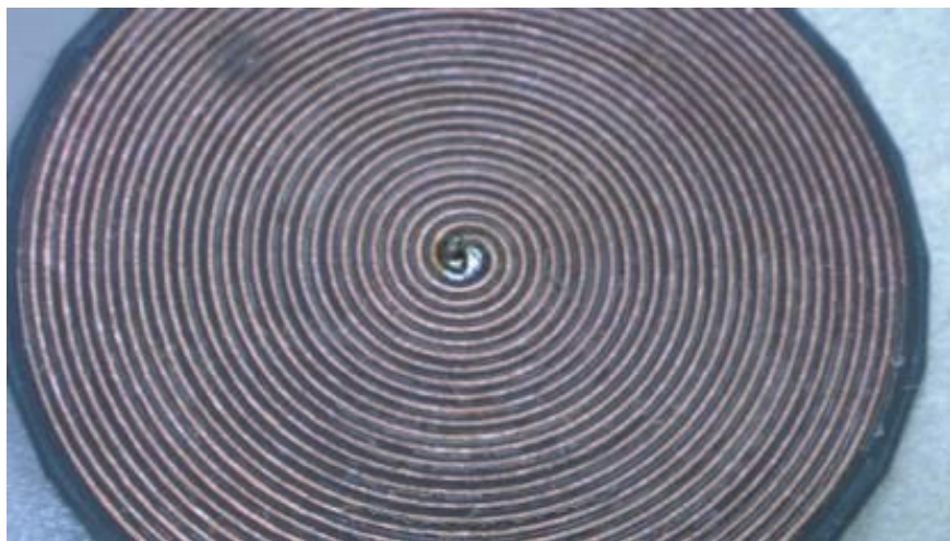
Figure 8.15: Fabricated spiral antenna with solder joints.
