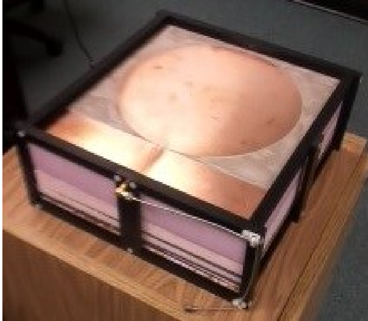
Figure 8.1: Manufactured UWB antenna over stacked EBG structure, along with Coax cable for feeding the antenna.
