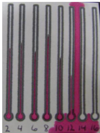
Figure SI. 4.4. Wax-printed paper channels (1.2 mm channel width, 0.3 mm wax walls, and 3 mm sampling spots, original printed side up in a Petri dish) typically contained amaranth solutions up to a volume of 12 \mu L.
