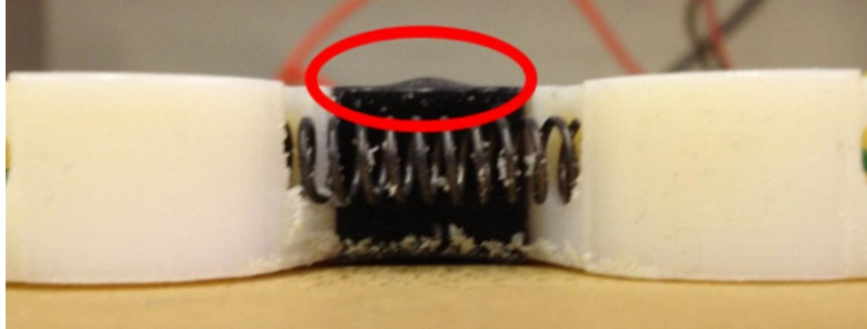
Figure 5.14. Out-of-Plane Bulging in Compliant Joint
