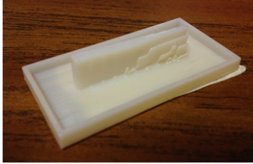
Figure 3.15. Stalagmites Denote a Non-Self-Supporting Angled Face
