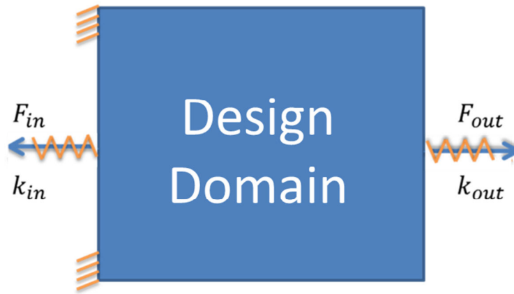
Figure 2.4. Design Domain and Loading for Inverter Case Study
