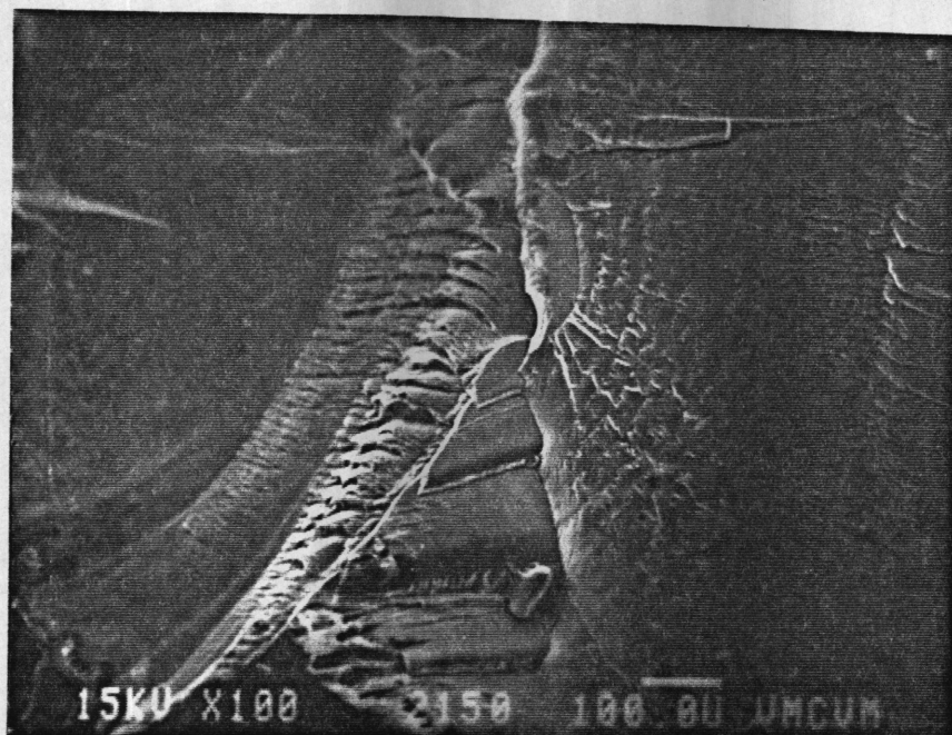
Figure 5. 59. Fusion Study of DHP dry blend by SEM (1/8 inch dia. die) at turn 17.: Leading edge (top), Trailing edge (bottom). Mag. 100
