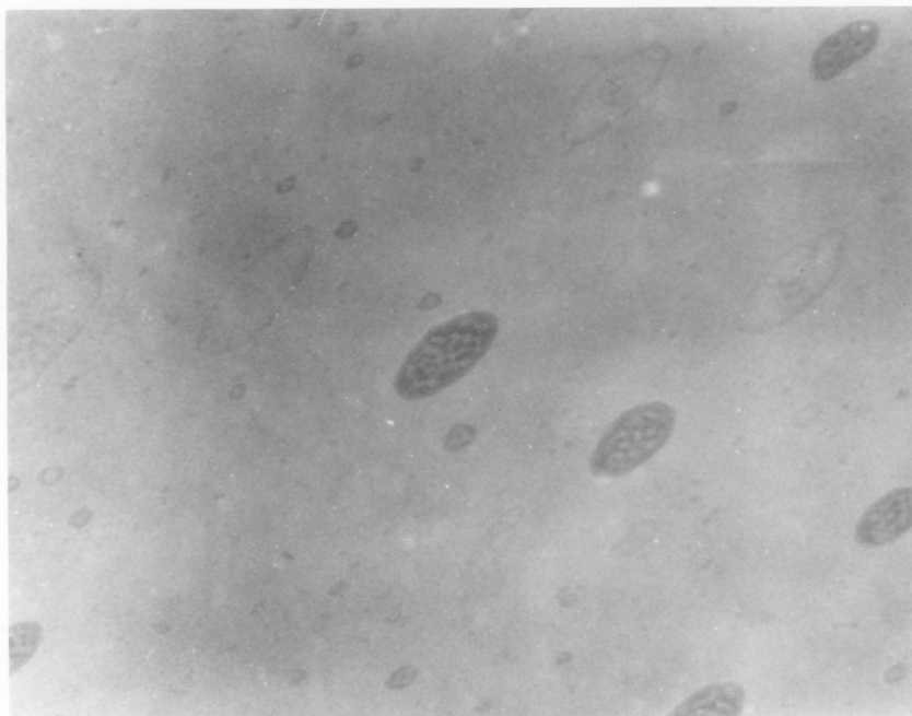
Figure 37. TEM micrograph of PSF(4900)/PSX(4400) block copolymer blended (0.5 wt.% PSX) with homopolysulfone.
