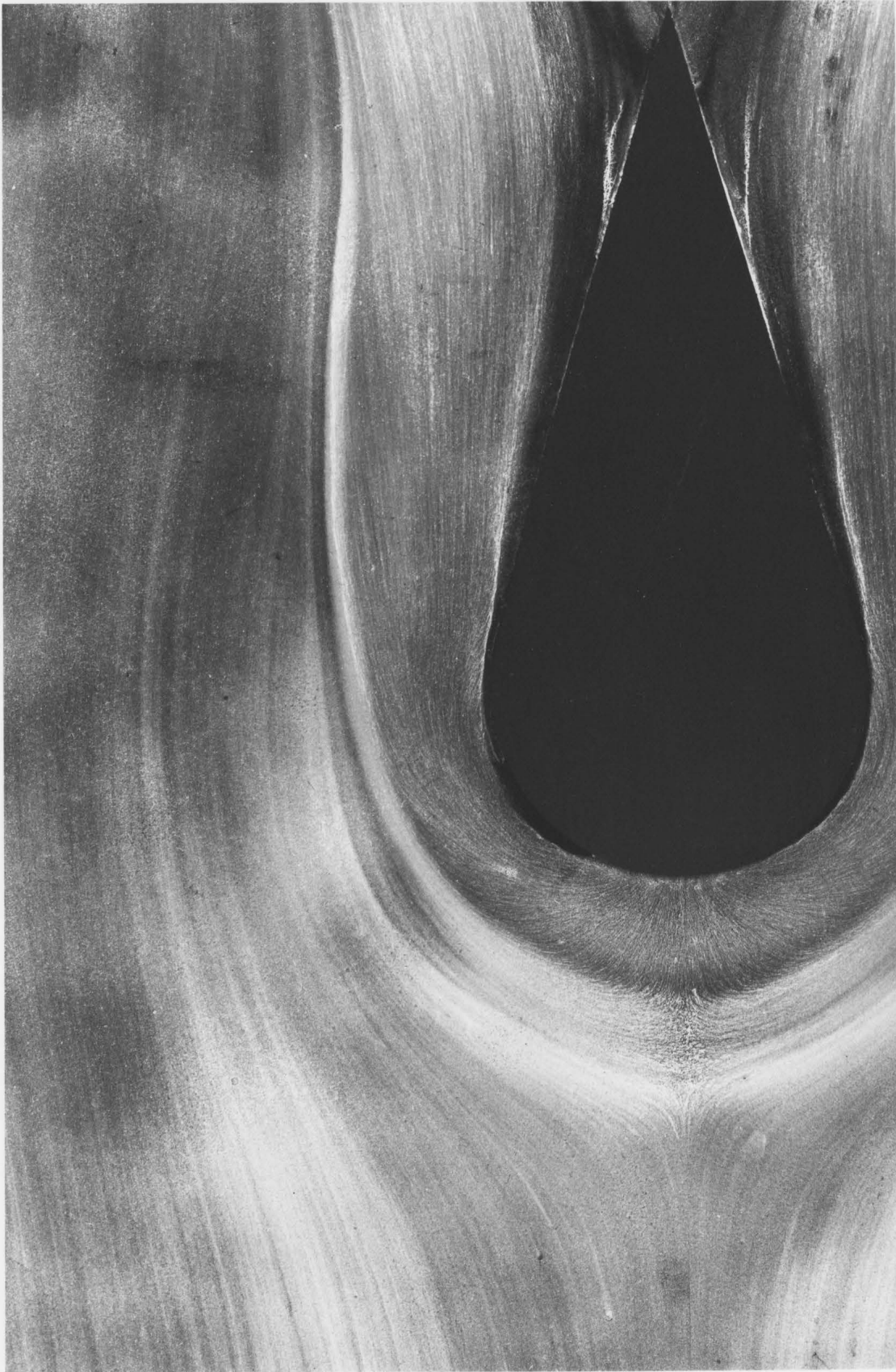
Fig. 4.9 Enlarged View of the Surface Flow Visualization on the Flat Floor of the Wind Tunnel
