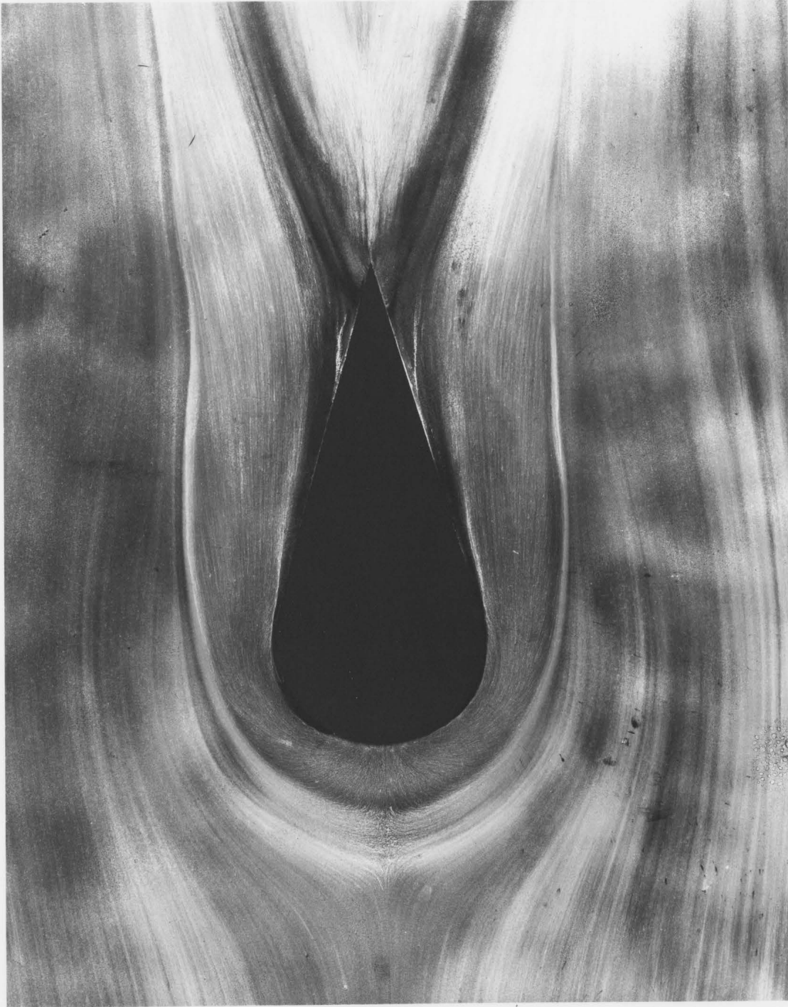
Fig. 4.8 Surface Flow Visualization on the Flat Floor of the Wind Tunnel
