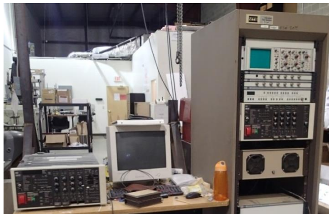
Figure 10.6 MTS 458.20 hydraulic control for 2-post rig
