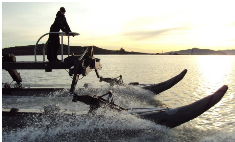
Figure B.1 Calm water testing in San Francisco, CA with WAM-V remotely operated from chase boat
