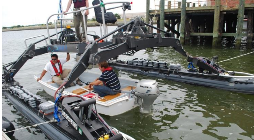
Figure A.2 WAM-V being prepared for water inclining test
