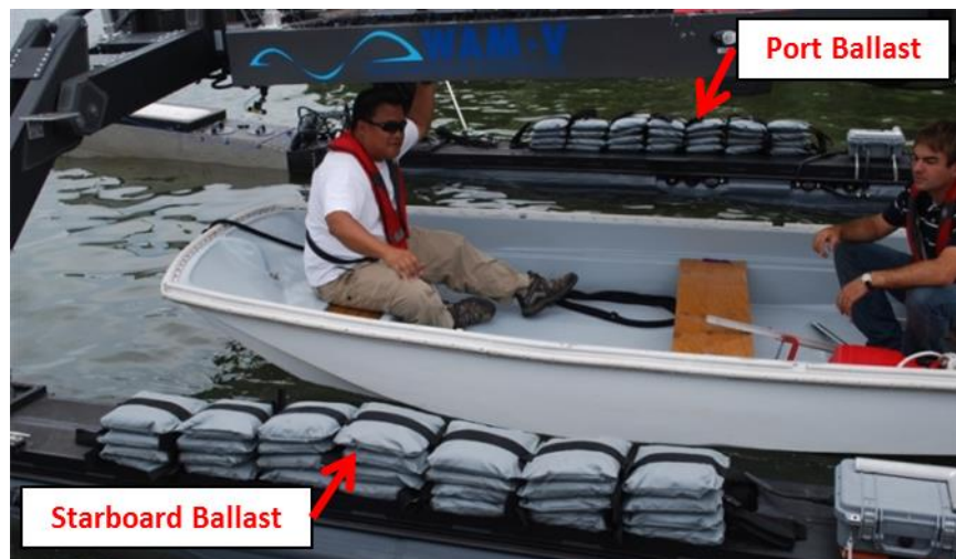
Figure A.3 Neutral location of ballast for water inclining test
