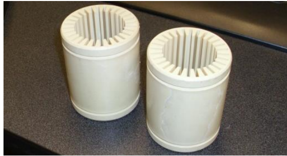
Figure 5.12 1.5 inch PTFE bearings used for rig (8 total bearings used on Quarter-Boat rig)
