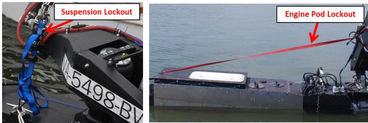
Figure A.4 Locked out suspension and engine pod for inclining tests
