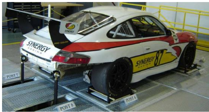
Figure 10.2 8-post shaker rig [76]
