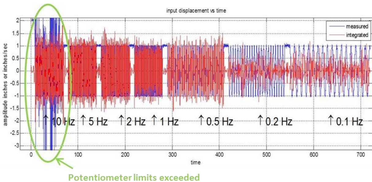
Figure 4.38 2 inch displacement multi-frequency test displacements
