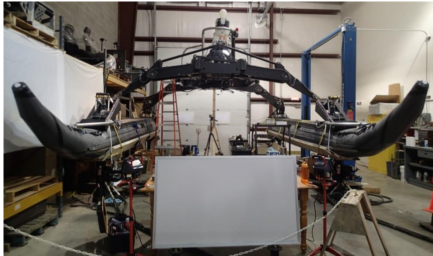
Figure 10.4 33-ft WAM-V on the 2-post testing rig
