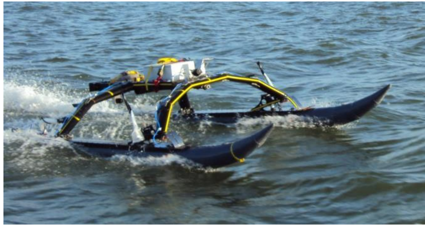
Figure 4.1 12-ft USV WAM-V
