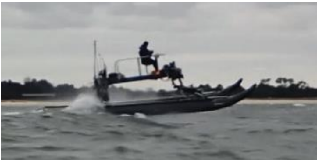
Figure 7.18 33-ft WAM-V during winter rough water testing (second generation suspension)
