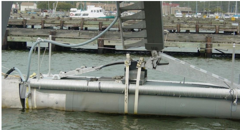
Figure 3.5 Rear suspension system assembly (shown locked out)
