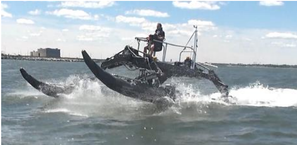
Figure 7.17 33-ft WAM-V during summer rough water testing (original suspension)
