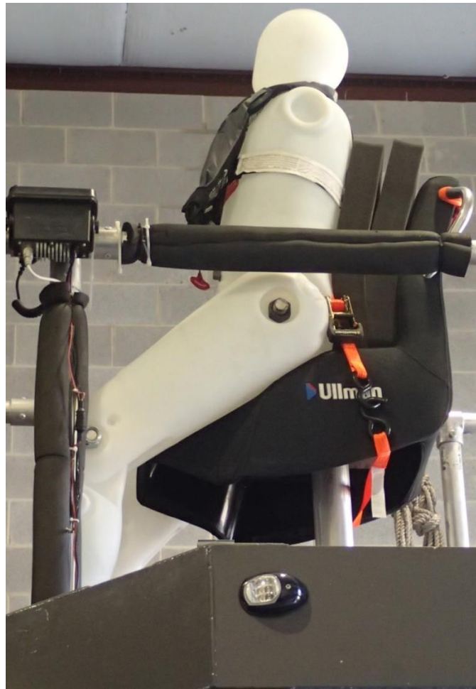
Figure 10.8 Operator dummy (BART) used for 2-post testing
