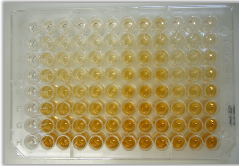
Figure 2-33: A 96-well microtiter plate used for performing a human anti-IgG, double antibody sandwich ELISA. 106 The deeper the color of the well is, the higher the antigen concentrations are.
