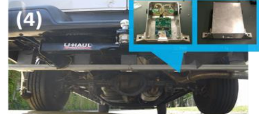
Surface radar array (5 sensors)
