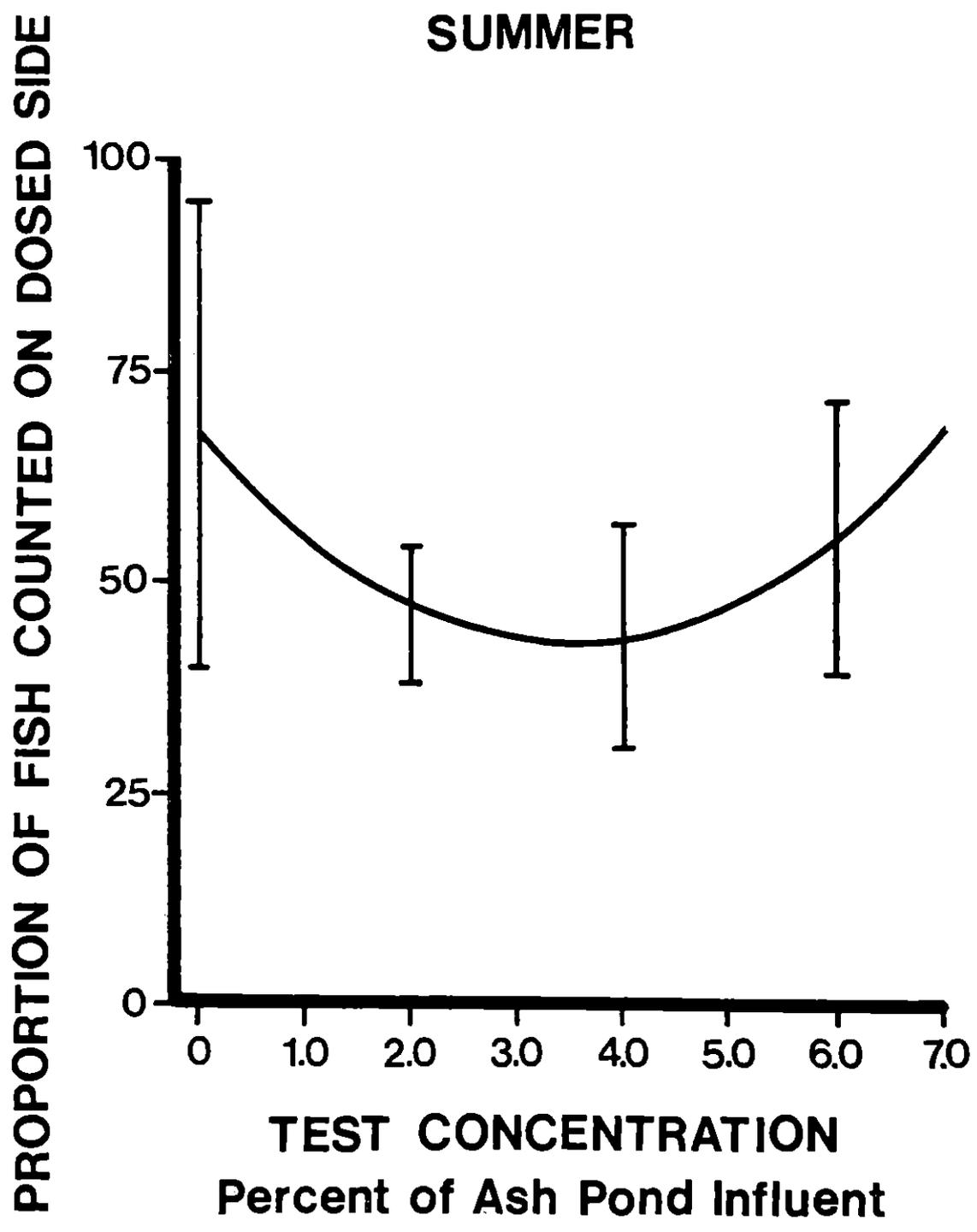
Figure 10. Avoidance response of fathead minnows to a blend of four metals following 3 (summer), 6 (fall) and 9 (winter) months of exposure to a concentration equal to 2% of the concentrations found in a fly ash basin influent. Test concentrations are expressed as test concentration plus background exposure. Vertical bars show 95% limits of quadratic regression.
