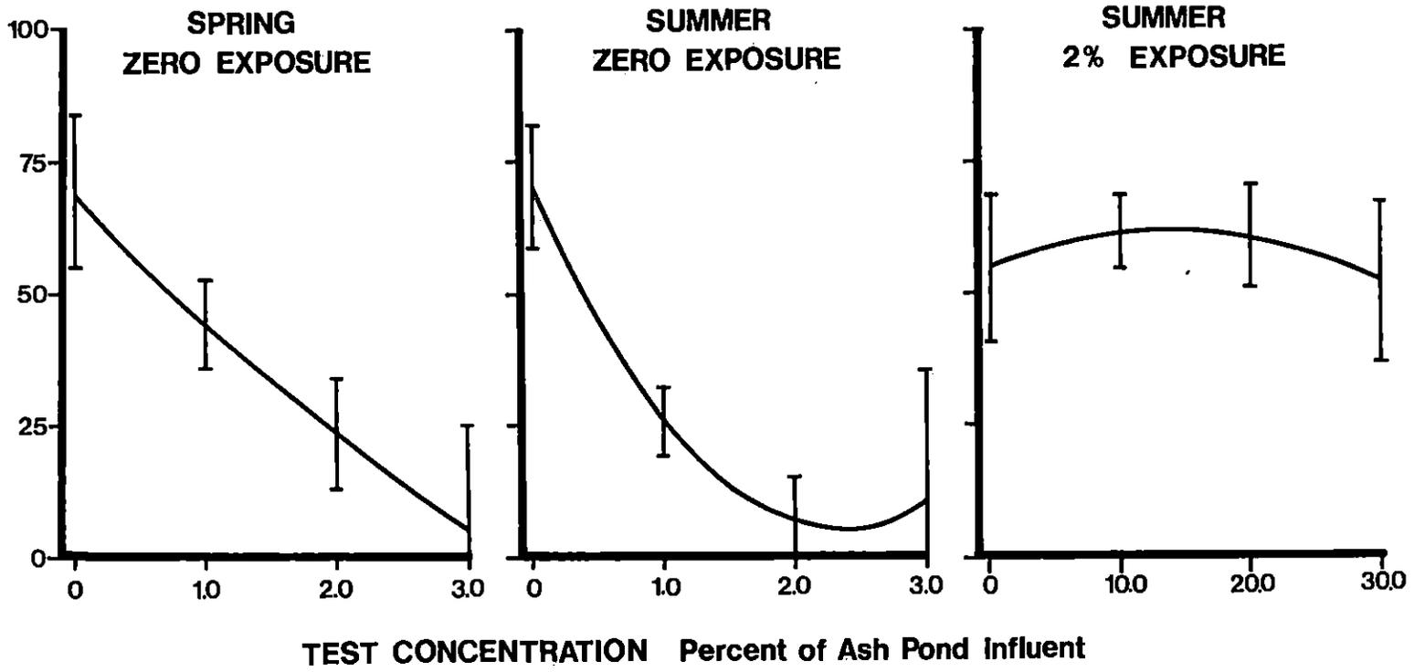
Figure 12. Avoidance response of fathead minnows in Adair Run to a blend of four metals. Zero exposure fish are control fish maintained in unaltered New River water for 3 months. High exposure fish were exposed in New River water to a metal blend concentration equal to 2% of concentrations found in a fly ash basin influent for 5 months. Test concentrations are expressed as test concentrations plus background exposure. Vertical bars show 95% confidence limits of quadratic regression.
