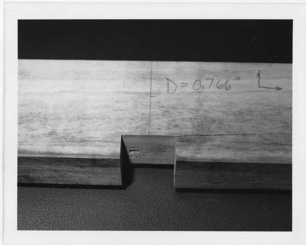
Figure 17. Unfilleted notch, after testing. This notch was machined with a radial arm saw using the method described in Section 4.2.3.2, page 80. Imperfections in notch shape away from the corners had no effect on crack initiation or propagation.
