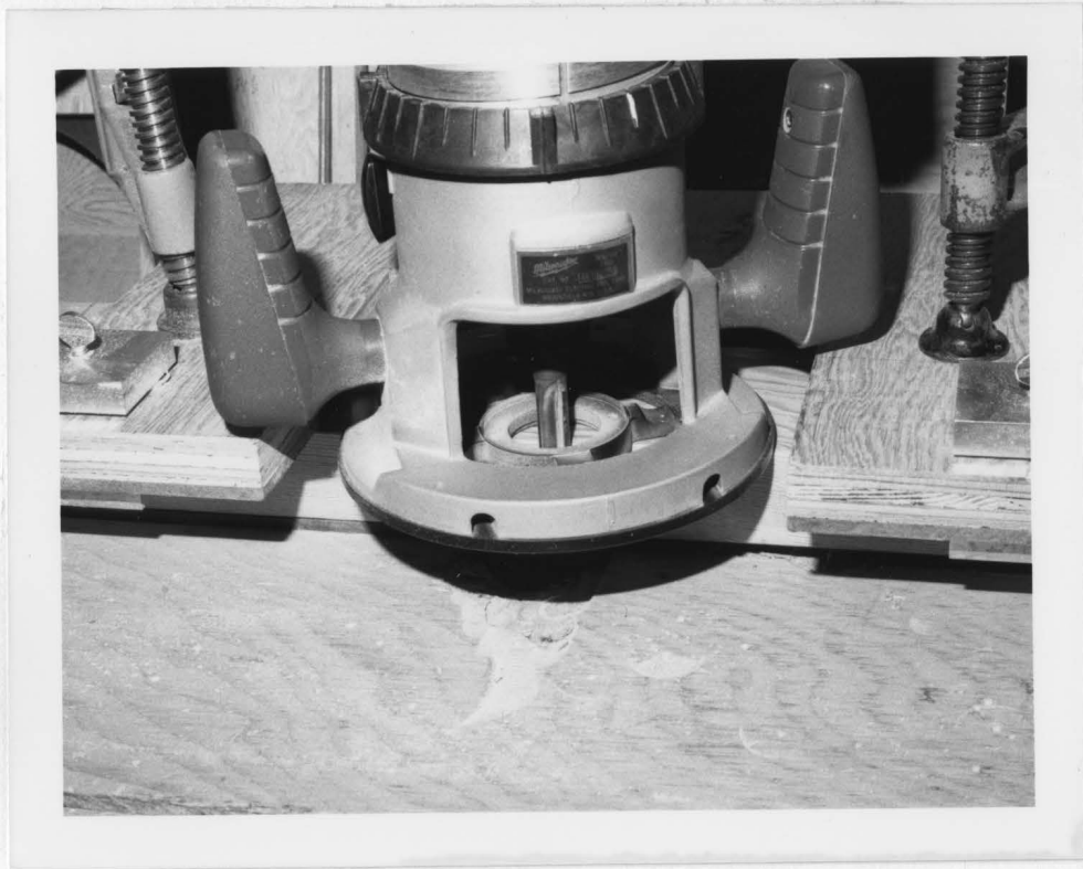
Figure 14. The router in position for finish machining of a pre-notched beam.
