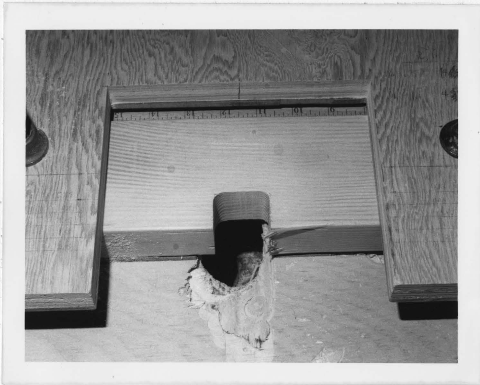
Figure 15. The beam of Figure 13, after finish machining. The chipping-out of the lower right (outer) notch corner is inconsequential due to low stress in that area.
