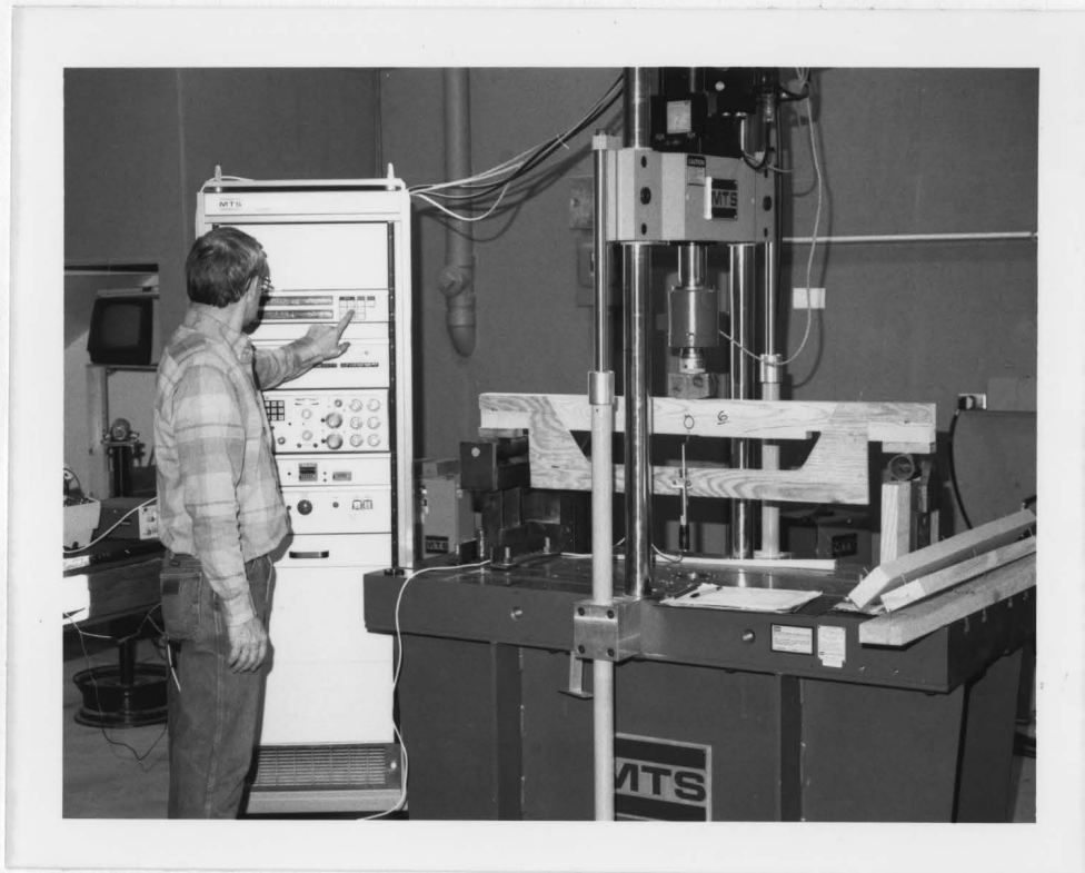
Figure 18a. Test rig for bending tests using servohydraulic universal testing machine. Overall view, including control console and chart recorder.
