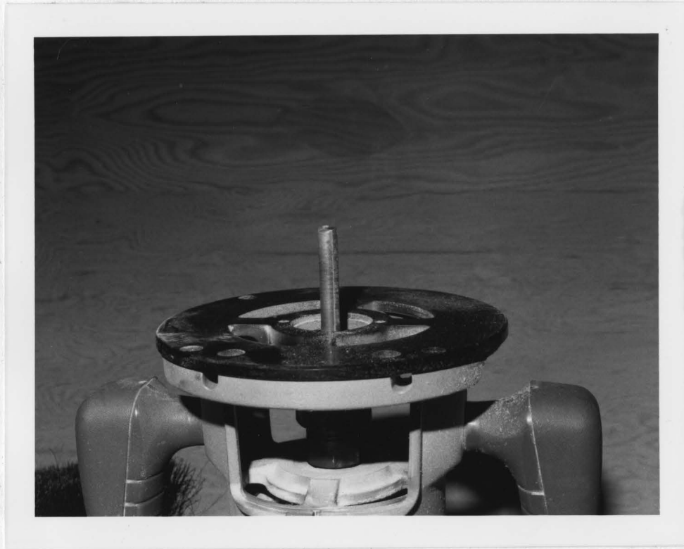
Figure 9. The router and carbide double-fluted straight bit used to machine notches for studies A and B. The circular router base, from which the bit protrudes, rests on the workpiece during machining.
