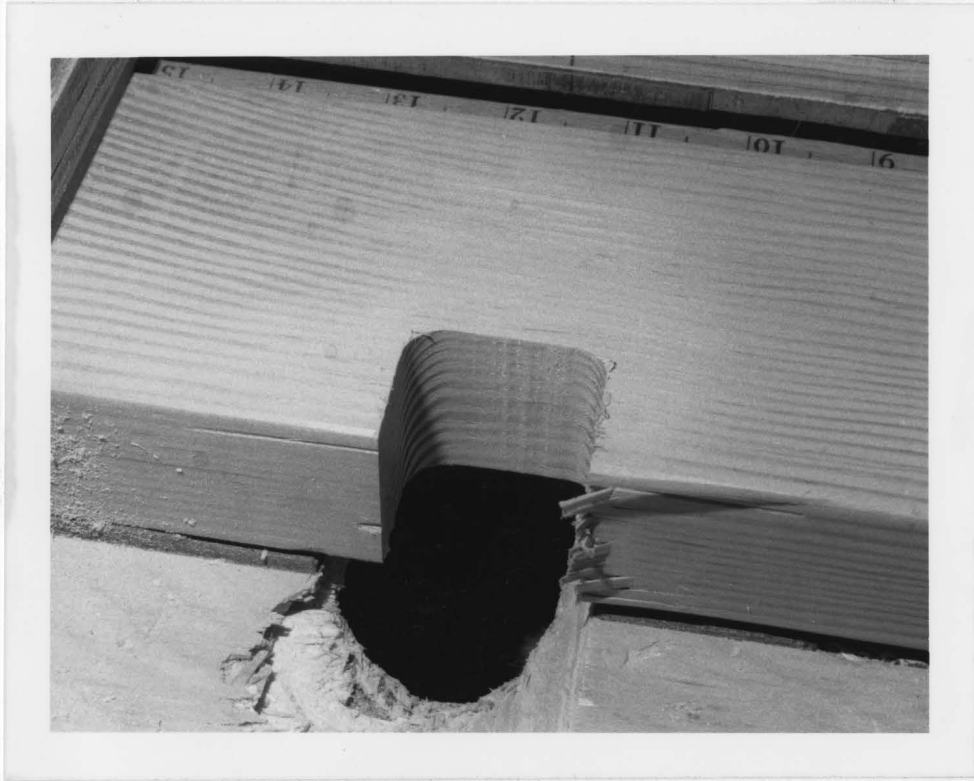
Figure 16. Magnified view of the notch of Figure 15. Note the smooth machined surface, particularly in the fillet regions which govern failure.
