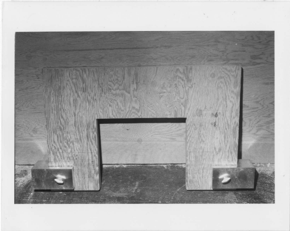
Figure 10. A template used to guide the router base for machining notches. The radius and length of the template cutout and the radii of the router bit and router base determine the radius of the notch fillet. The metal clamps set the notch depth.
