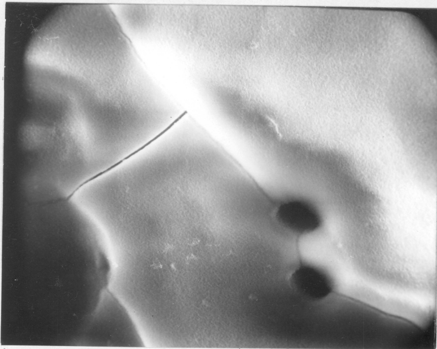
FIGURE 8. CRACK IN OXIDE COATING. 4300X
