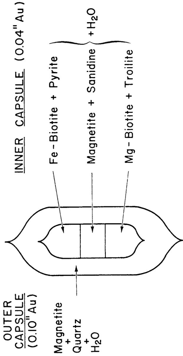
Figure 1. Schematic of capsule arrangement showing the three layers, outer capsule and their constituents.
