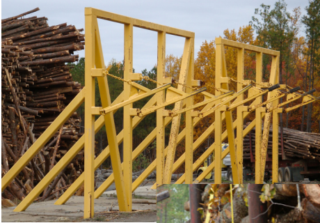
Figure 14. Unbinding rack at mill
