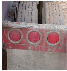
Figure 11. Lights obscured by dirt and mud
