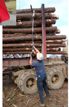
Figure 9. Using a pole saw to trim a load
