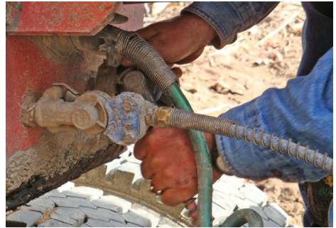
Figure 13. Checking glad hands and electrical connections before entering public roads
