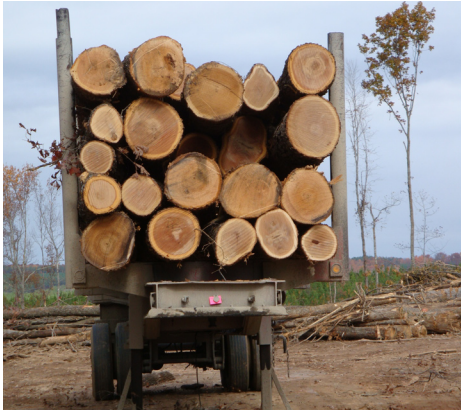
Figure 7. Load height lower than bolsters
