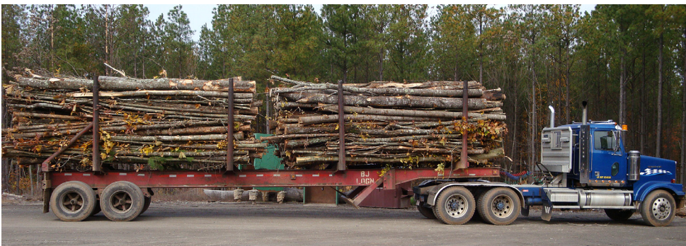
Figure 11. Common tractor trailer configuration with a 4-bolster log trailer.
