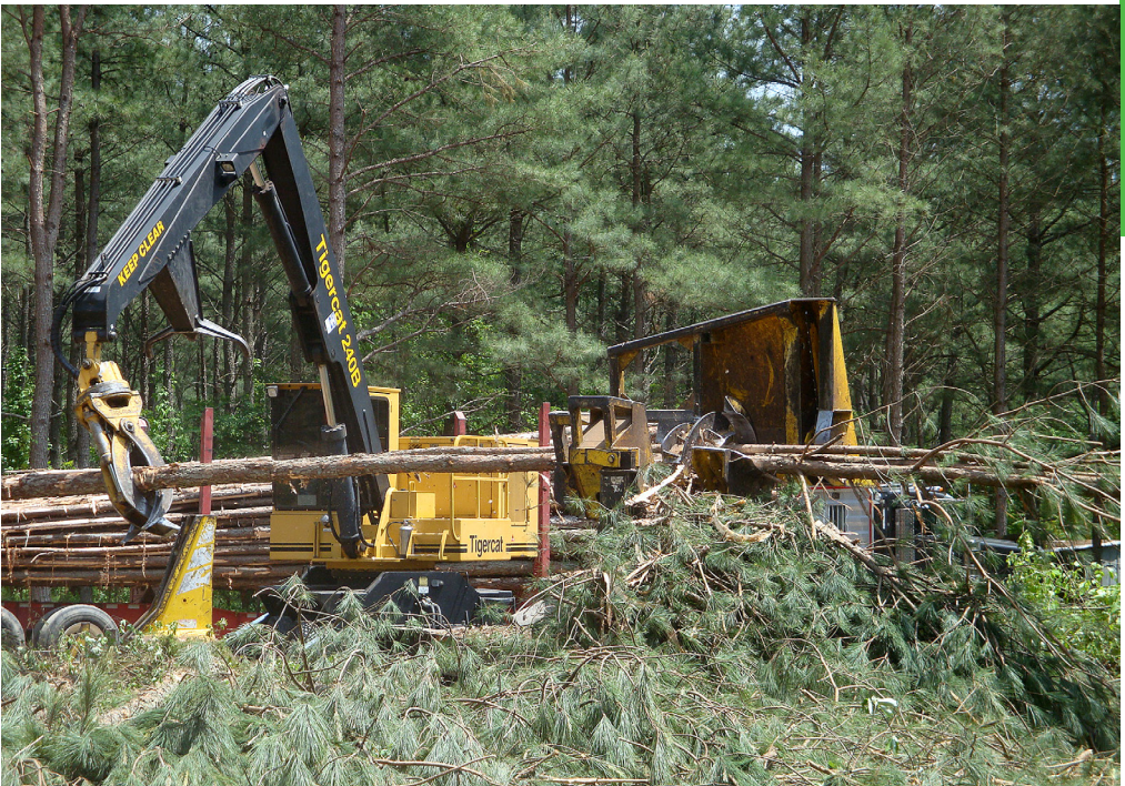
Figure 8. Knuckle boom loader delimiting at the landing using a pull-through delimitter.
