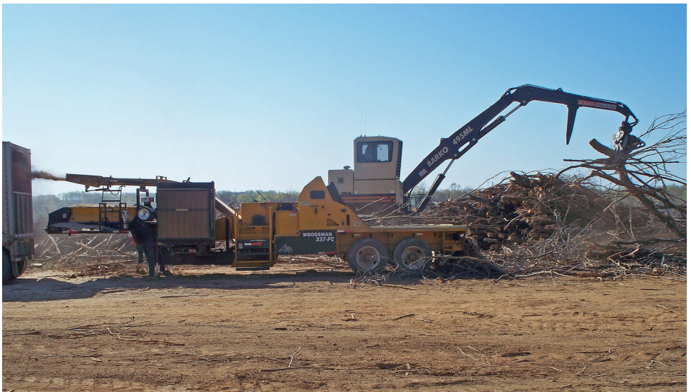
Figure 10. Whole tree chipper, producing dirty chips from logging residue.
