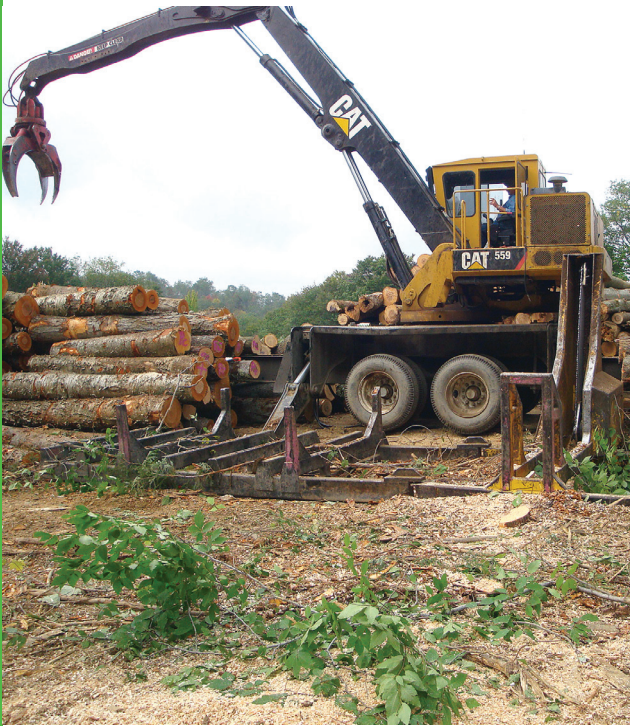
Figure 9. Buck saw, also referred to as slasher saw.
