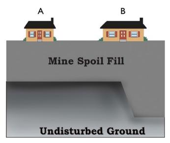
Figure 1. Settlement of underlying mine spoils can affect buildings constructed on mine spoil fills. The spoil depth under Building A (left) is relatively uniform, whereas Building B (right) is built over an area where spoil depth varies. Building B is more likely to be damaged due to differential settlement because of variations in the depth of the underlying spoils, and because it covers a larger lateral area.
