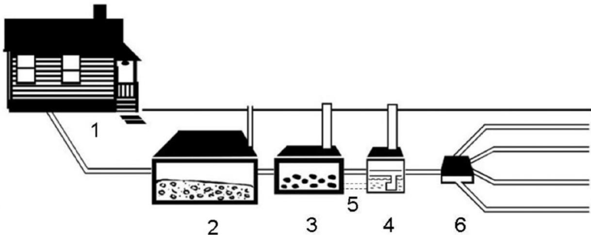
Figure 1. Recommended system design for on-site wastewater disposal systems for installation on existing mines (conceptual, not to scale).
