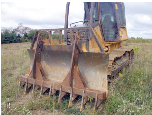
Figures 3a - c. Equipment that can be used for site clearing operations: (a, upper left) a “KG-style” shearing blade, attached to a dozer, for shearing dense woody vegetation at ground level; (b, lower left) a brush-rake, also attached to a dozer, for grubbing roots and moving and piling sheared vegetation with low disturbance of surface soils; and (c, upper right) a tree shredder, attached to a skid-steer tractor, for grinding and shredding both above-ground and below-ground stumps and roots, an operation that can prevent much of the vigorous re-sprouting that will occur if only woody tops are removed.
