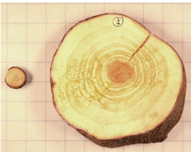
Figure 6. Cross-sections of 8-year-old white pine trees: left, growing on loose sandstone minesoils; right, growing on compacted shale minesoil; left, growing on loose sandstone minesoils. Note: (Grid line spacing = 1 inch.)
