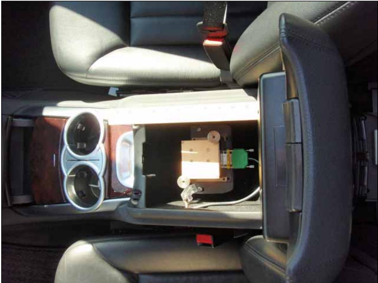
**Figure 34. Location of Crossbow Inertial Measurement System in Mercedes-Benz R350**
