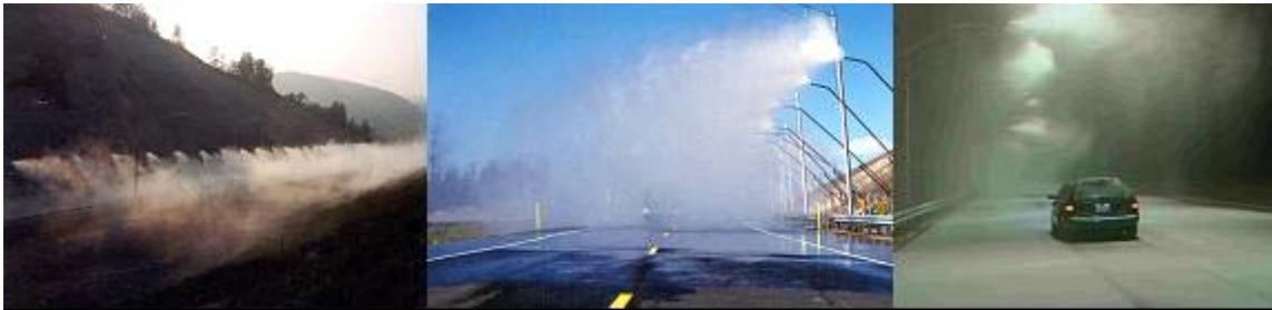
**Figure 56. Fog, rain, and snow equipment installed on the Smart Road.**
