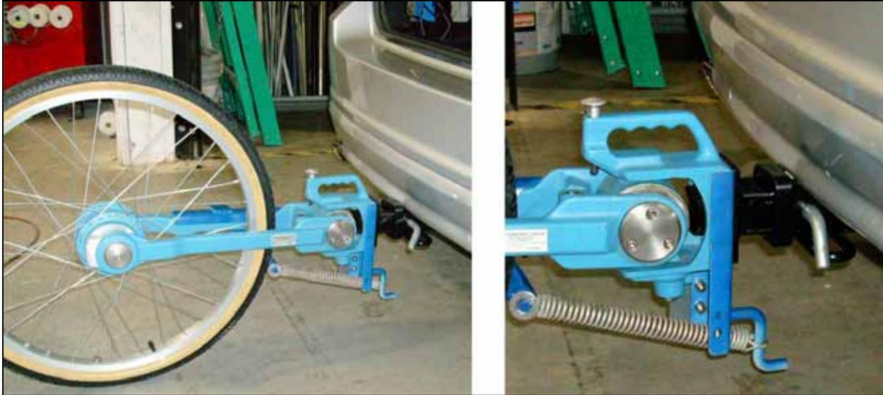
**Figure 28. Fifth Wheel and Hitch Setup on the Volvo S80**
