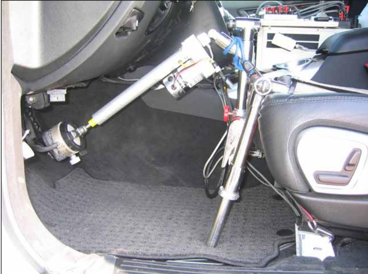
**Figure 12. Brake Controller Mounted to the Driver Seat and Brake Pedal**
