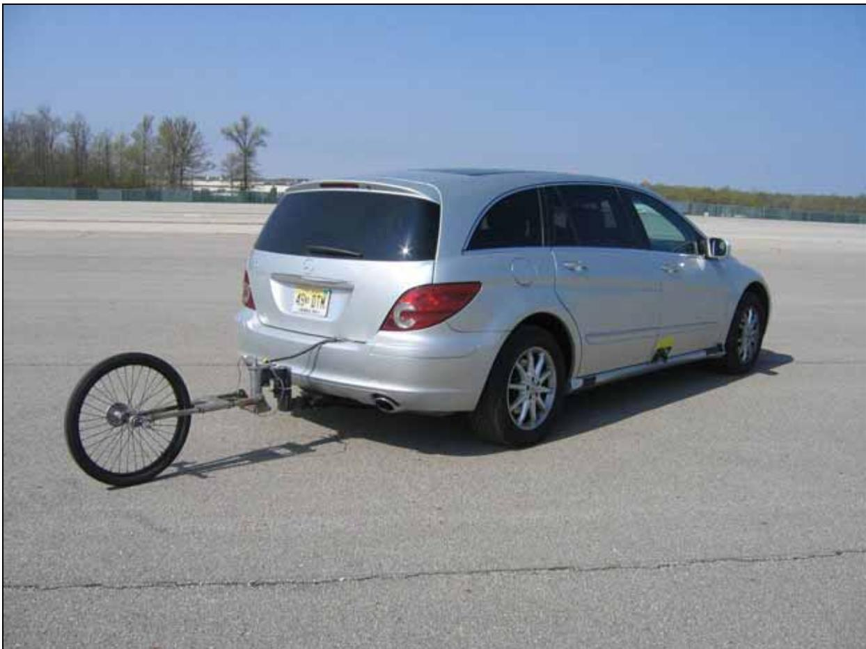
**Figure 13. Position of Fifth Wheel on the Mercedes-Benz R350**
