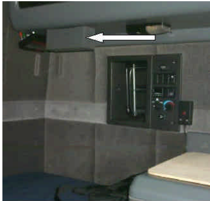
Figure 9. Acoustically transparent microphone enclosure located above the bed in the Volvo sleeper berth.
