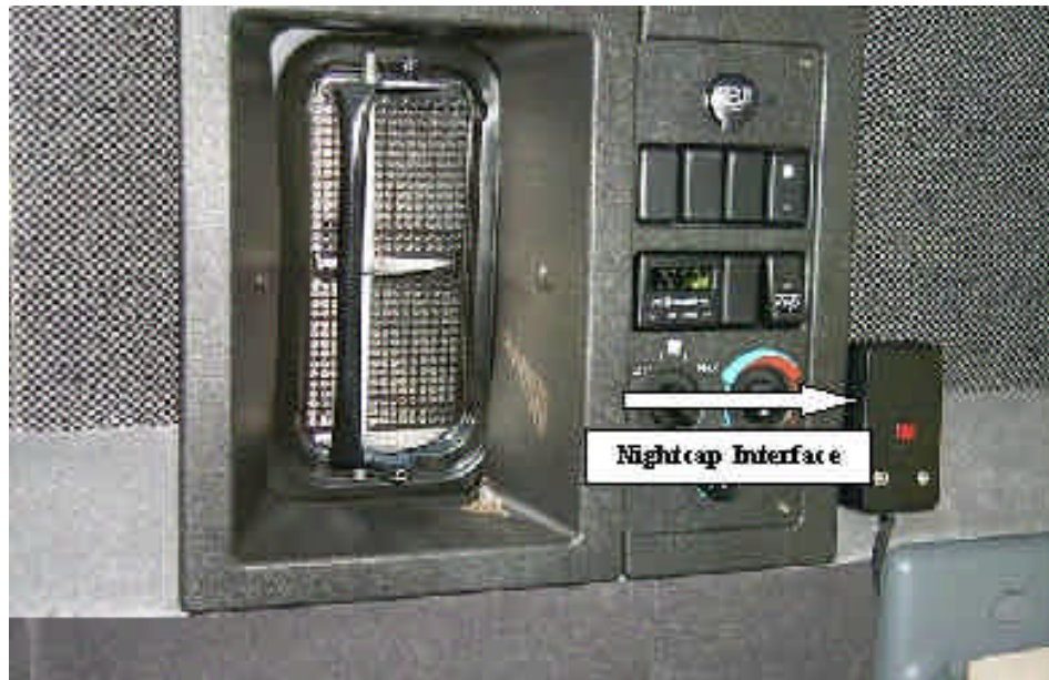
Figure 12. Nightcap interface unit located in the Volvo sleeper berth.
