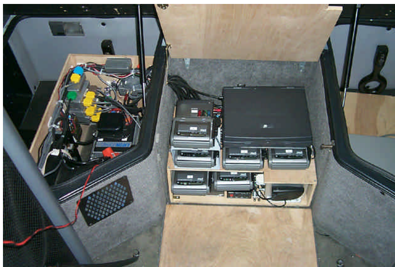
Figure 3. Instrumentation concealed under the bunk in the Volvo. Access was gained from inside the sleeper berth by lifting the mattress platform.
