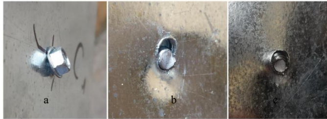
Fig. 10. Failure modes for 5454 group a. Ply 1- front b. Ply 1 – back c. Ply 2- front
