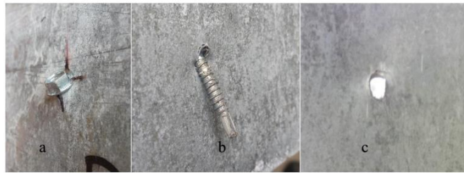
Fig. 8. Failure modes for 4343 group
