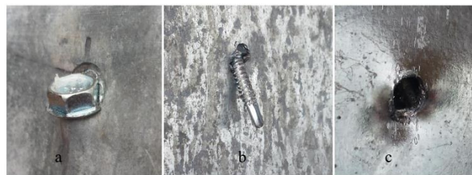
Fig. 18. Failure modes for 4354 group a. Ply 1-front b. Ply 1 – back c. Ply 2-back
